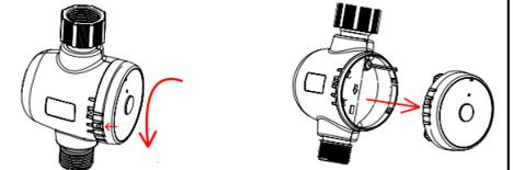
a. Rotate the front panel
