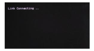
8) The system will spend 20-30 seconds constructing the link, depending on link strength and the signal channel condition. When wireless link is established the RSSI light will illuminate, indicating the current wireless signal strength, VIDO indicators will light, and the connected HD monitor will be playing the real-time video and audio.
