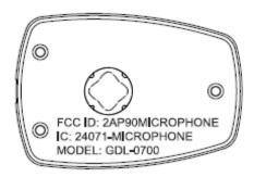
The label will be etched onto the Microphone Assembly Case. The case measures 1.813" by 1.25" by 0.438" thick.
