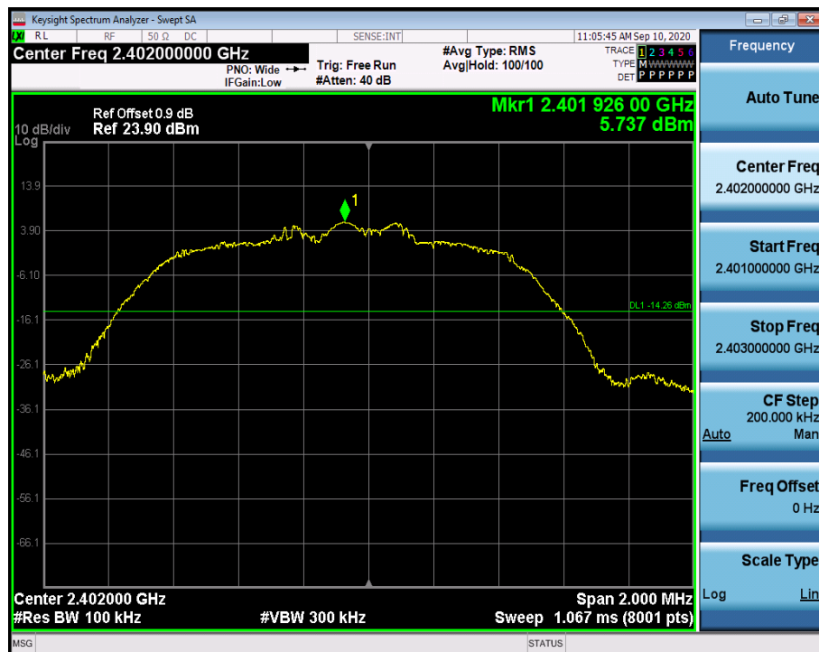
RF Conducted Spurious Emissions_2DH5_2402
