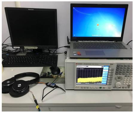
Conducted Emissions at AC Power Line (150kHz-30MHz) Test Setup
