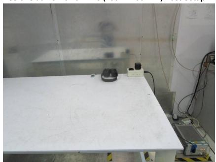
Radiated Emissions which fall in the restricted bands & Radiated Spurious Emissions Test Setup
