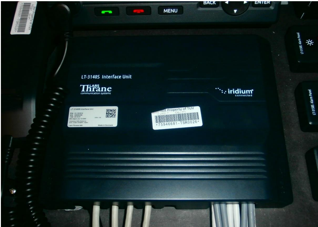
Figure 1.5.3 Interface unit (Top)
