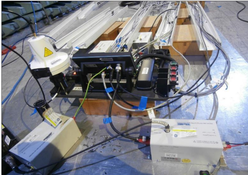
Figure 20 - Test Setup - 150 kHz to 80 MHz
