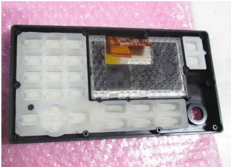
Internal view – display module and keypad membrane
