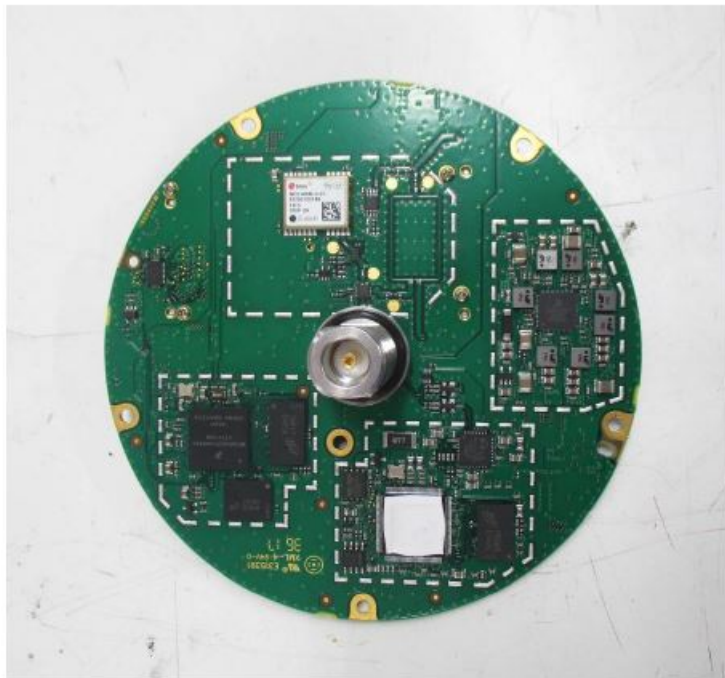
Internal view – antenna, power and radio PCB, underside
