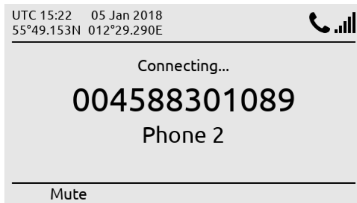
Figure 28: LT-3110 Control Unit – voice call connecting...
