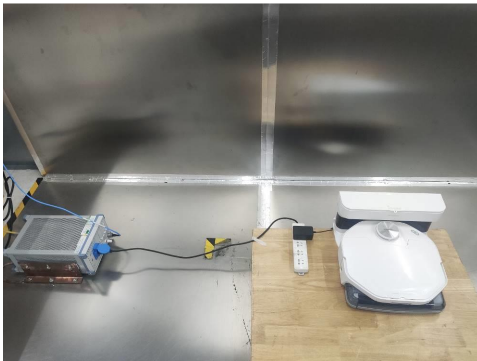
Photograph 3: Set-up photo for Conducted Emission
