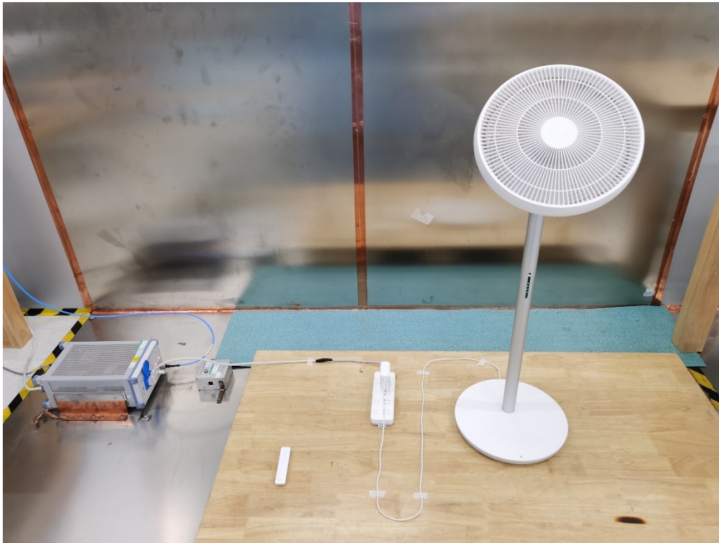
Photograph 3: Set-up for Conducted Emission on AC Mains
