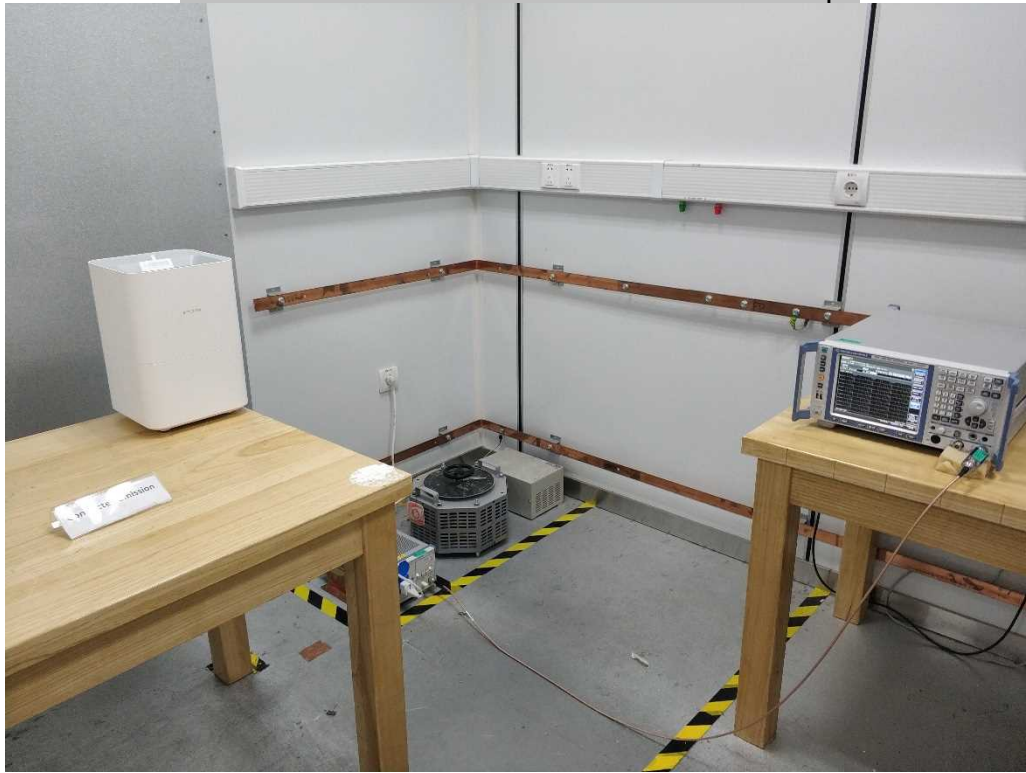
Radiated Emission test setups 9kHz ~ 30MHz
