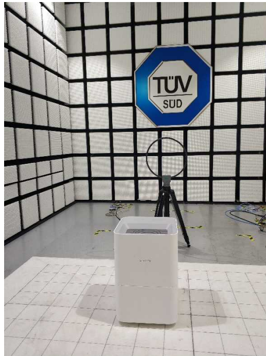
Radiated Emission test setups 9kHz ~ 30MHz
