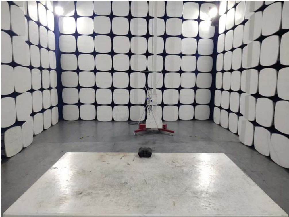
Test Setup Below 1GHz
