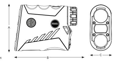
A – 3 in / 76 mm B – 4.3 in / 109 mm C – 1.4 in / 36 mm
