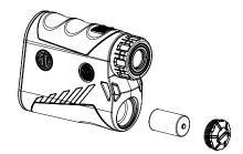
After installation of the battery and depressing the RANGE button, the status of the rangefinder is displayed:
