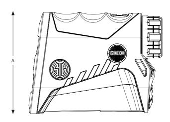
A – 2.9 in / 76mm B – 3.9 in / 107mm C – 1.4in / 33mm
