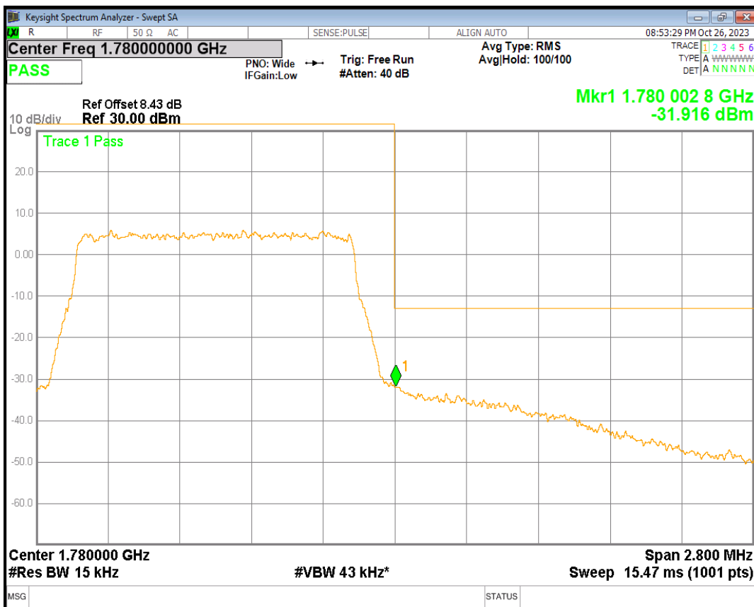
Band66 QPSK BW=10MHz Channel=132022 RB Size=50 Position=#0
