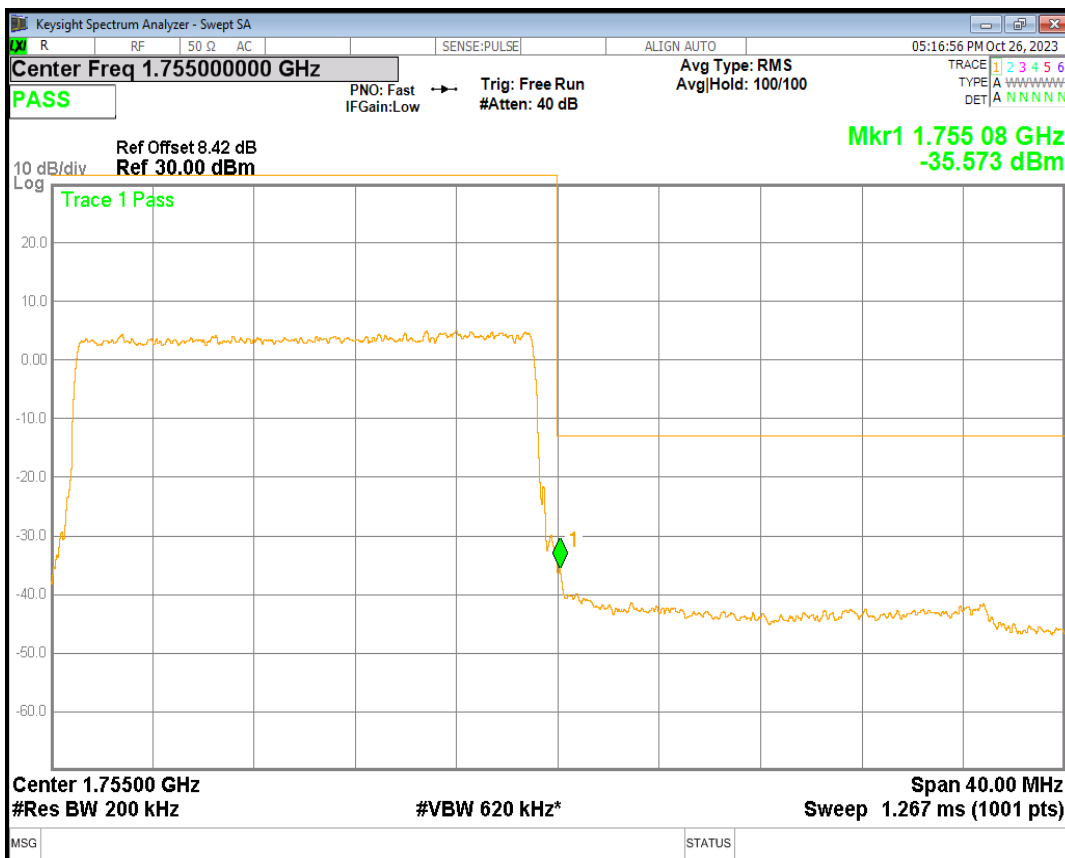
Band4 QPSK BW=3MHz Channel=19965 RB Size=15 Position=#0
