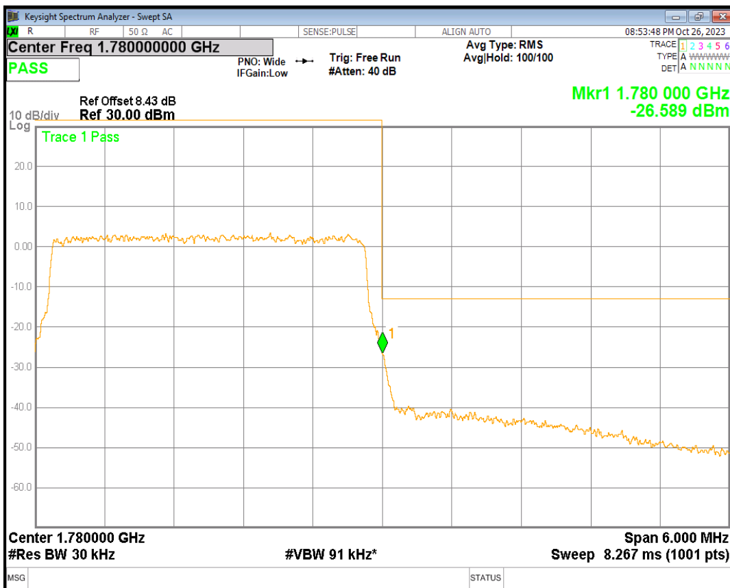
Band66 16QAM BW=5MHz Channel=131997 RB Size=25 Position=#0
