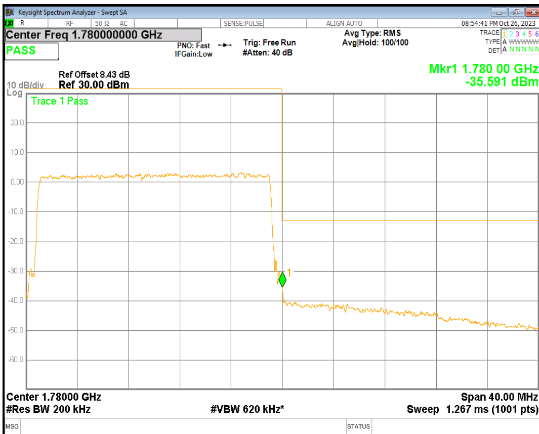
Band66 16QAM BW=3MHz Channel=131987 RB Size=15 Position=#0
