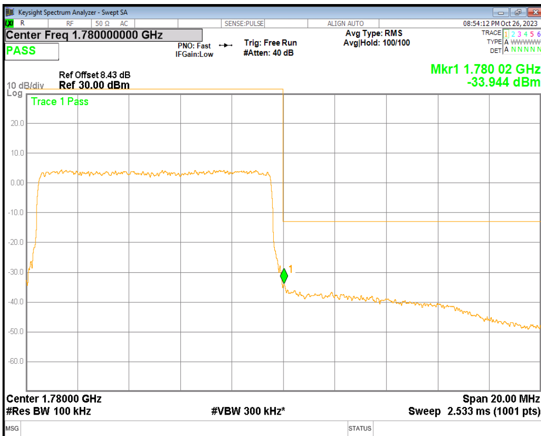
Band66 QPSK BW=15MHz Channel=132047 RB Size=75 Position=#0
