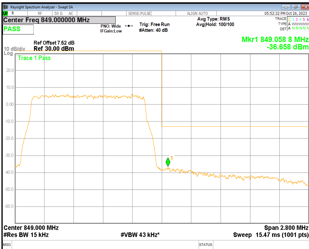
Band5 QPSK BW=10MHz Channel=20450 RB Size=50 Position=#0
