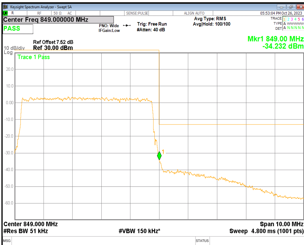
Band5 QPSK BW=1.4MHz Channel=20407 RB Size=6 Position=#0
