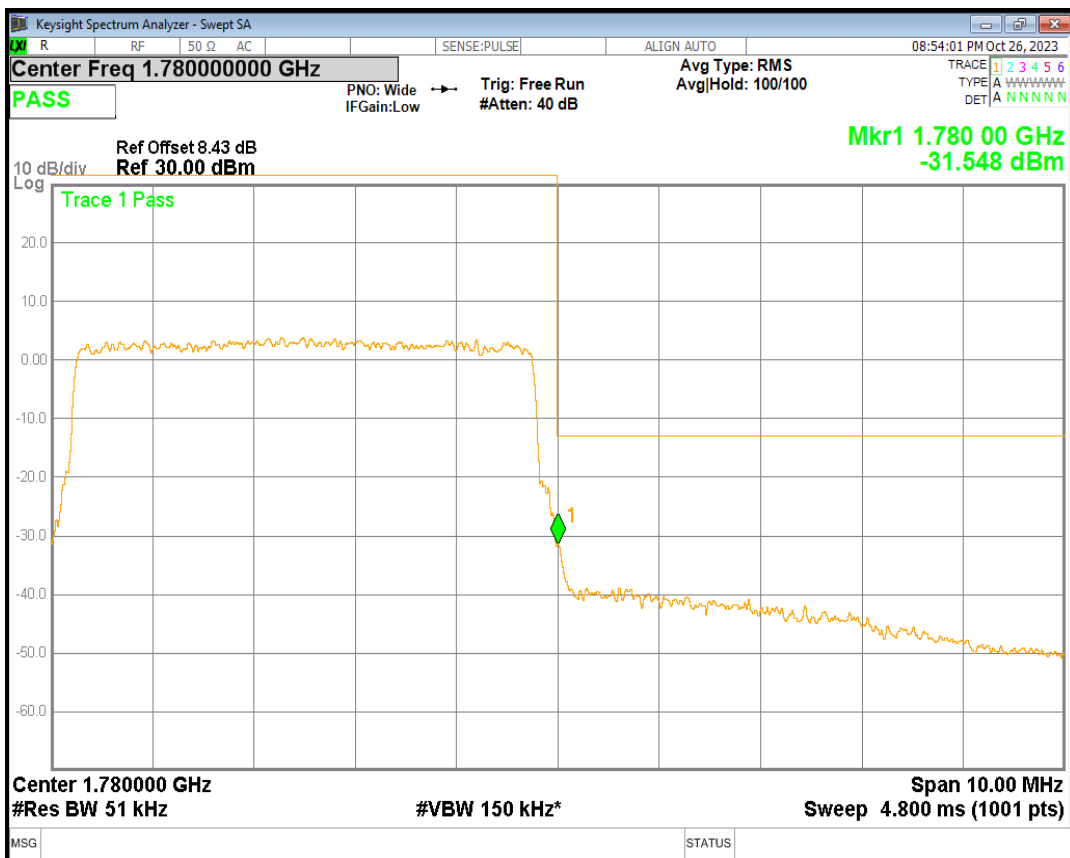
Band66 QPSK BW=1.4MHz Channel=131979 RB Size=6 Position=#0
