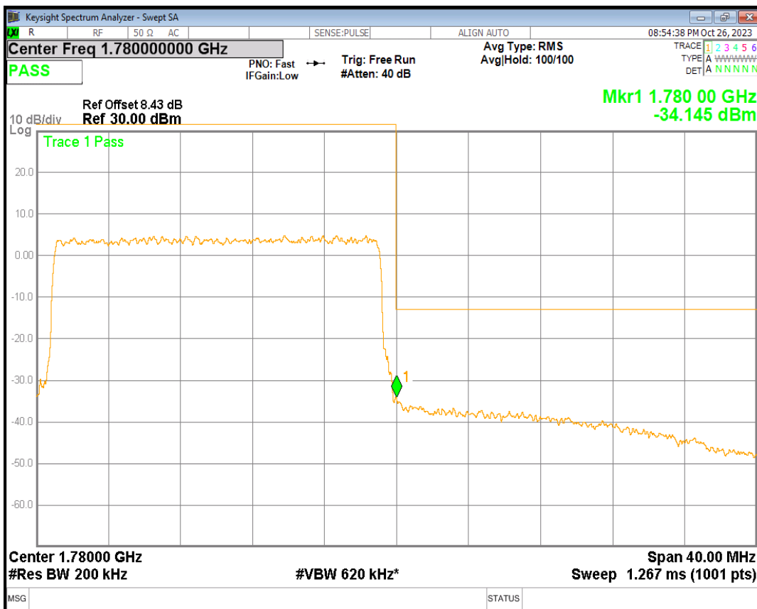
Band66 QPSK BW=3MHz Channel=131987 RB Size=15 Position=#0
