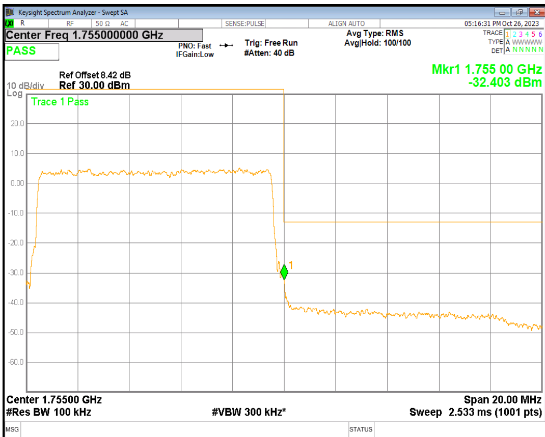
Band4 QPSK BW=15MHz Channel=20025 RB Size=75 Position=#0
