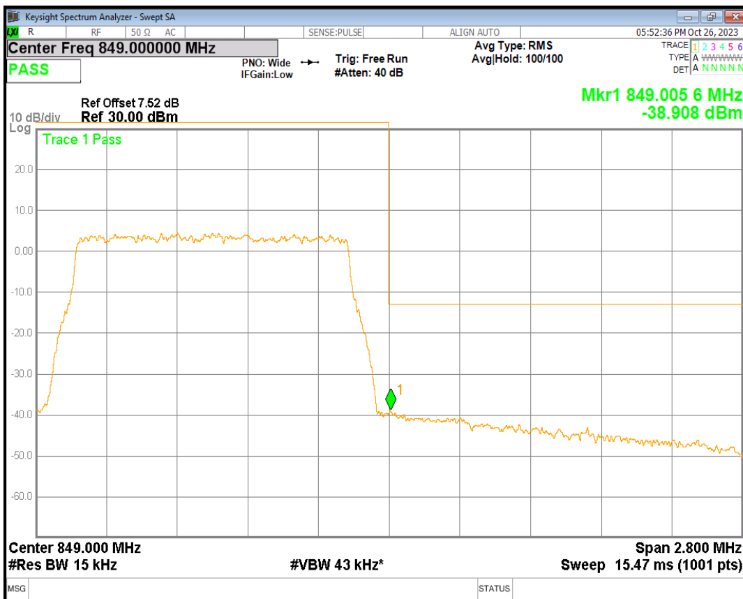
Band5 16QAM BW=10MHz Channel=20450 RB Size=50 Position=#0
