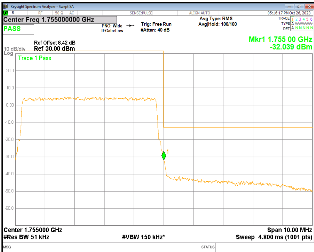
Band41 16QAM BW=10MHz Channel=39700 RB Size=50 Position=#0
