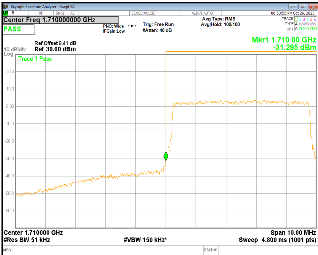
Band66 16QAM BW=5MHz Channel=132647 RB Size=25 Position=#0
