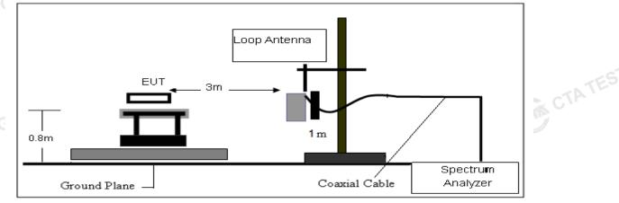
(B) Radiated Emission Test-Up Frequency 30MHz~1GHz
