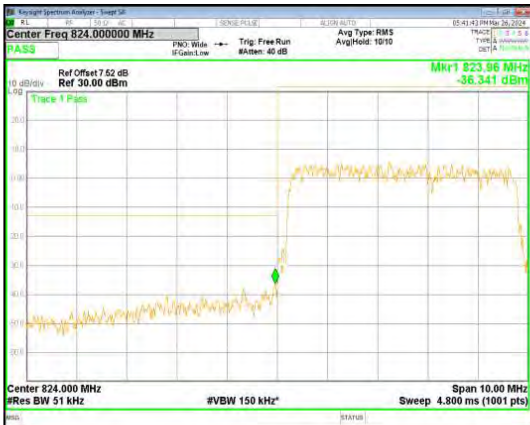
Band26(824-849) 16QAM BW=3MHz Channel=27025 RB Size=15 Position=#0
