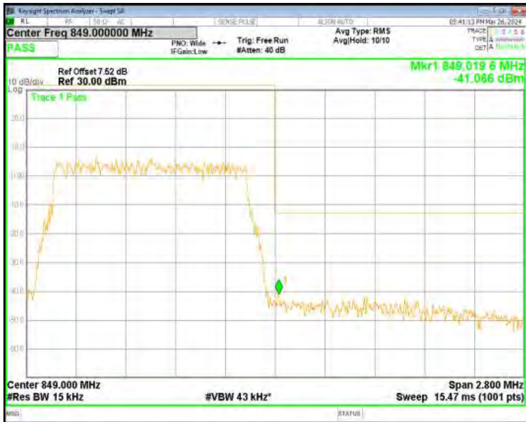
Band26(824-849) 16QAM BW=15MHz Channel=26865 RB Size=75 Position=#0
