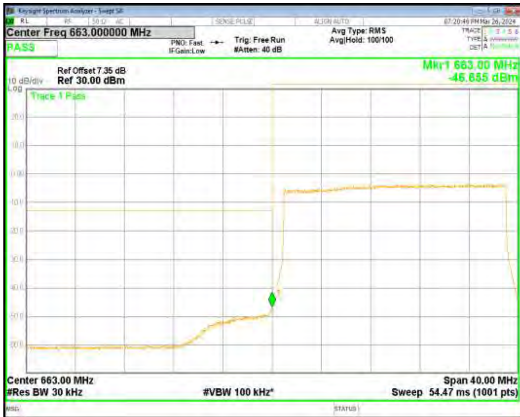
Band71 QPSK BW=20MHz Channel=133372 RB Size=100 Position=#0
