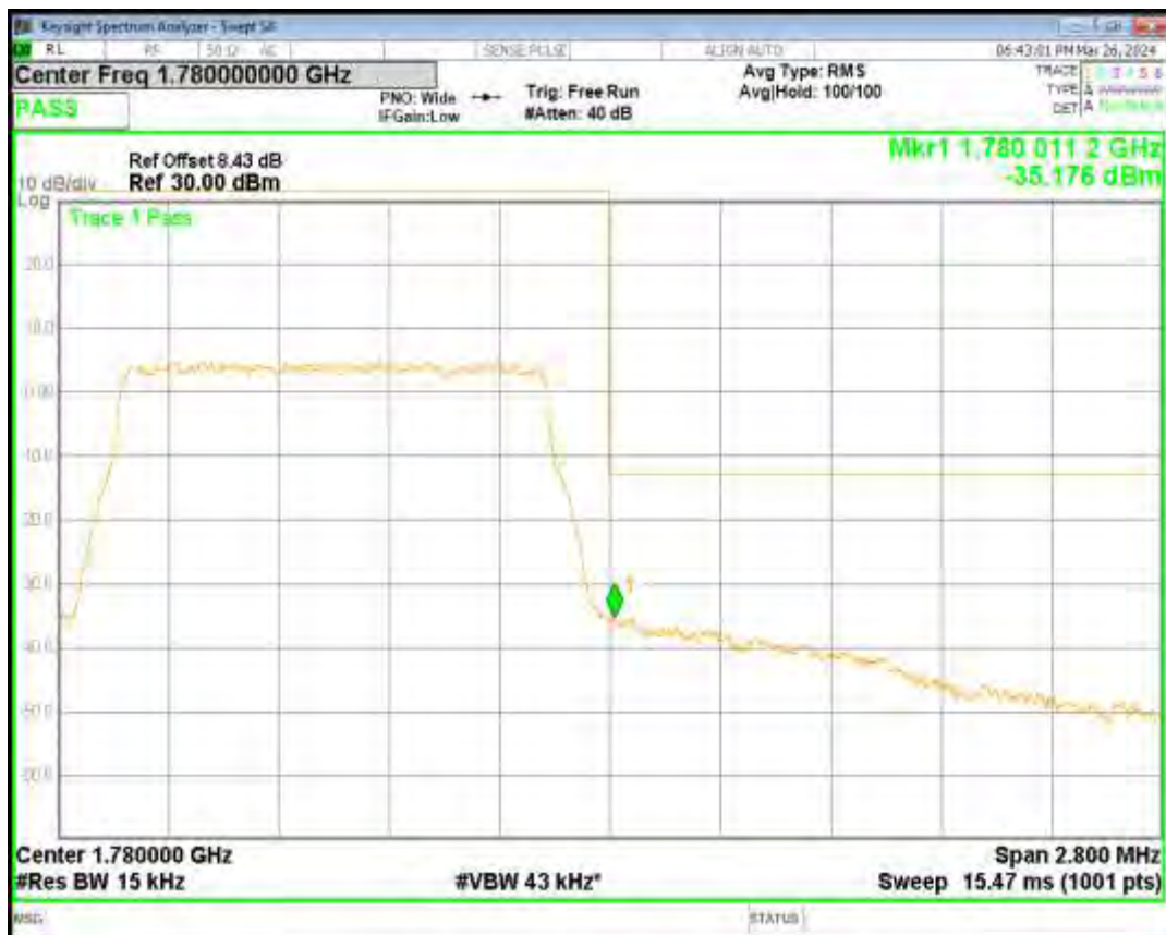
Band66 QPSK BW=1.4MHz Channel=131979 RB Size=6 Position=#0
