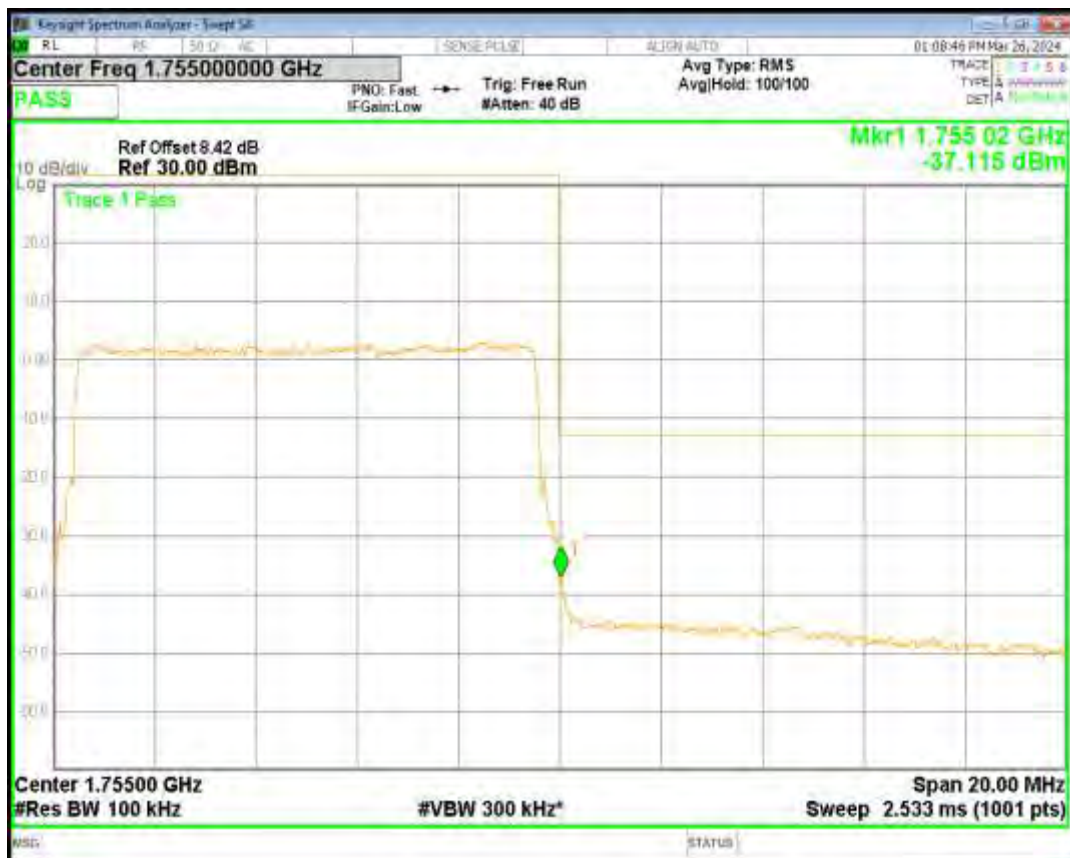
Band4 16QAM BW=15MHz Channel=20025 RB Size=75 Position=#0
