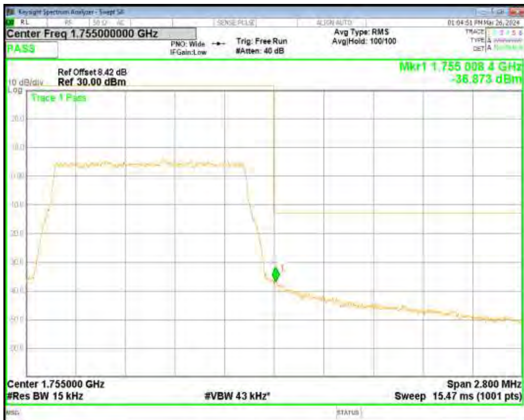
Band4 QPSK BW=10MHz Channel=20000 RB Size=50 Position=#0
