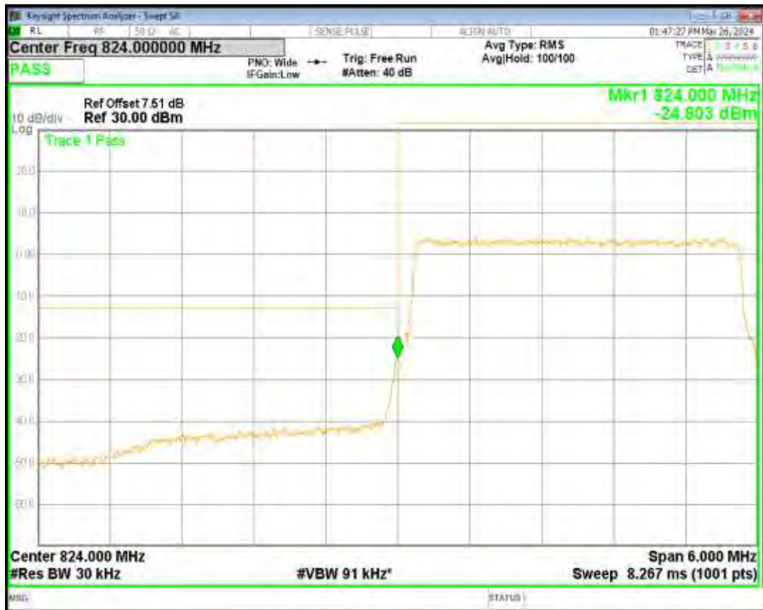
Band5 QPSK BW=3MHz Channel=20635 RB Size=15 Position=#0
