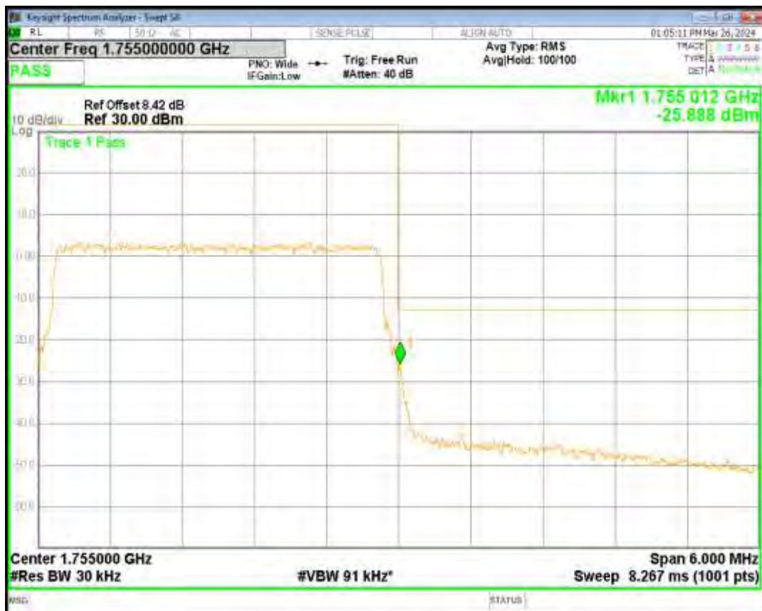
Band4 16QAM BW=5MHz Channel=20375 RB Size=25 Position=#0
