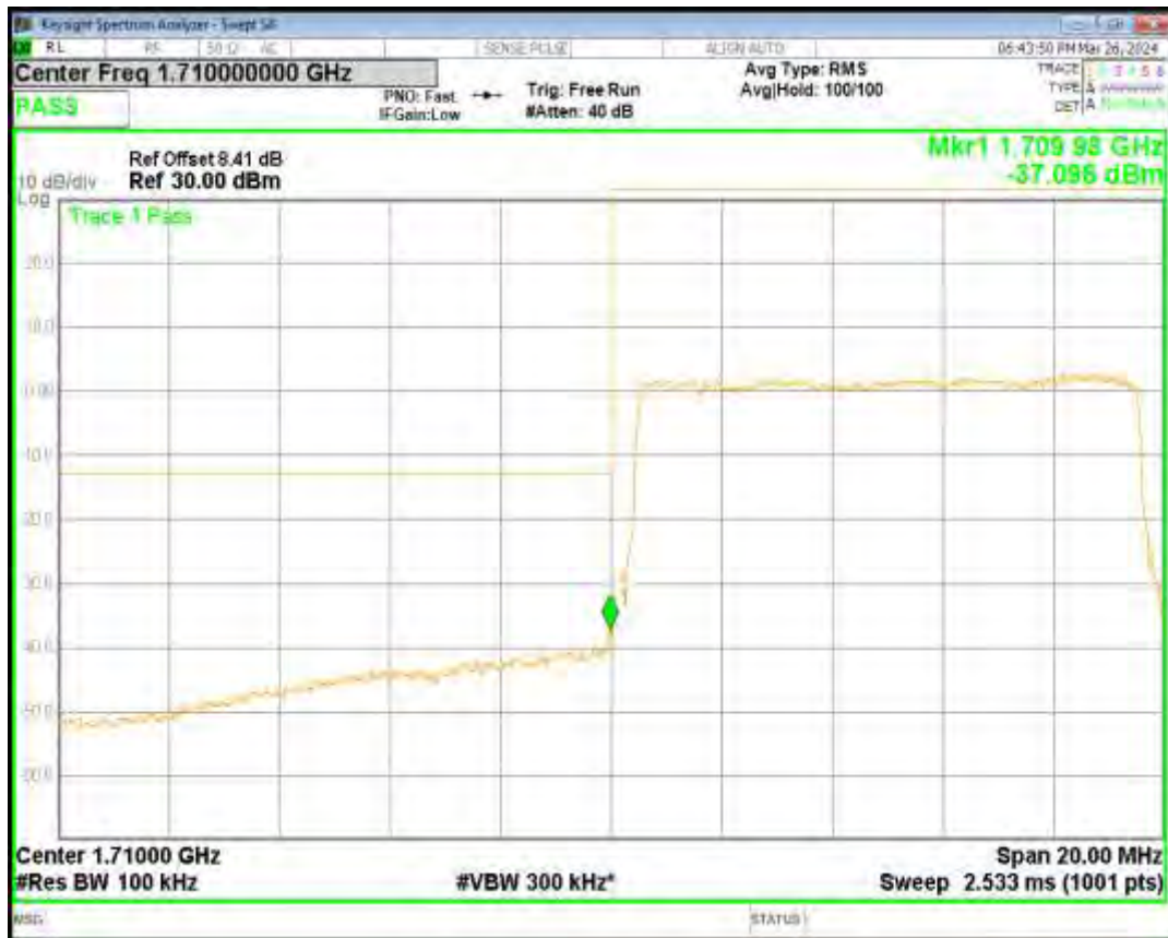
Band66 QPSK BW=10MHz Channel=132622 RB Size=50 Position=#0
