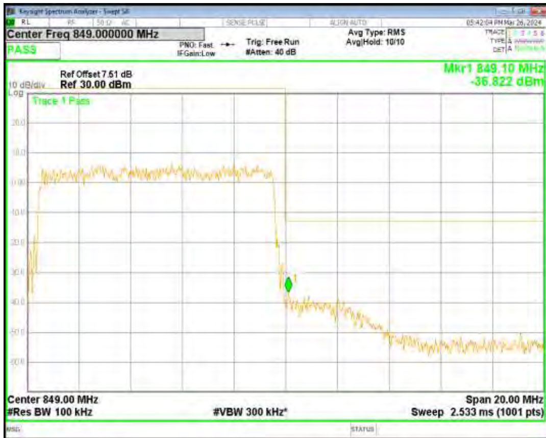
Band26(824-849) QPSK BW=15MHz Channel=26865 RB Size=75 Position=#0
