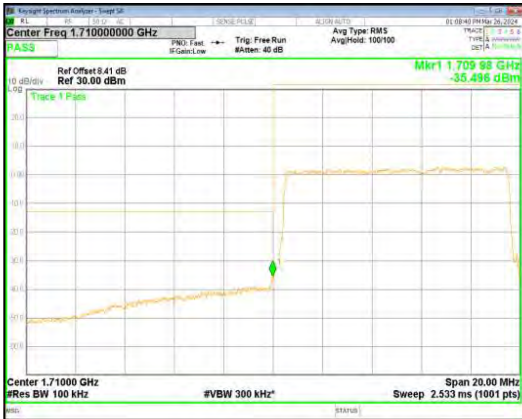
Band4 16QAM BW=10MHz Channel=20350 RB Size=50 Position=#0
