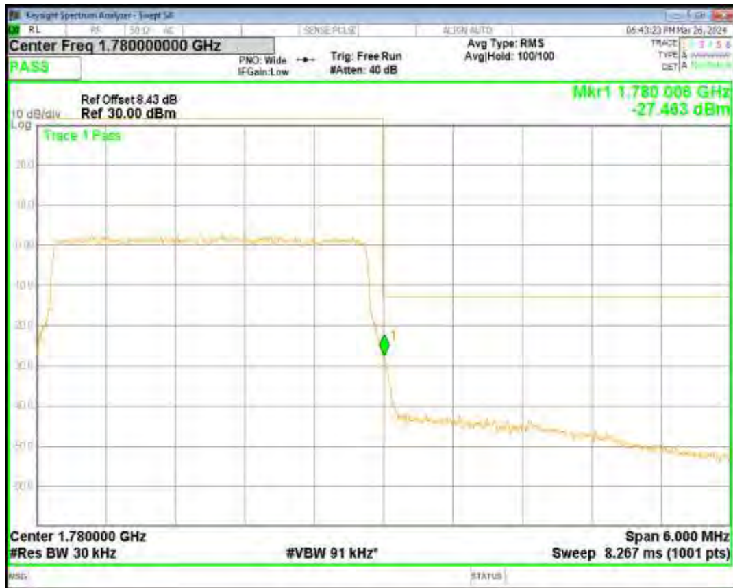
Band66 16QAM BW=5MHz Channel=132647 RB Size=25 Position=#0
