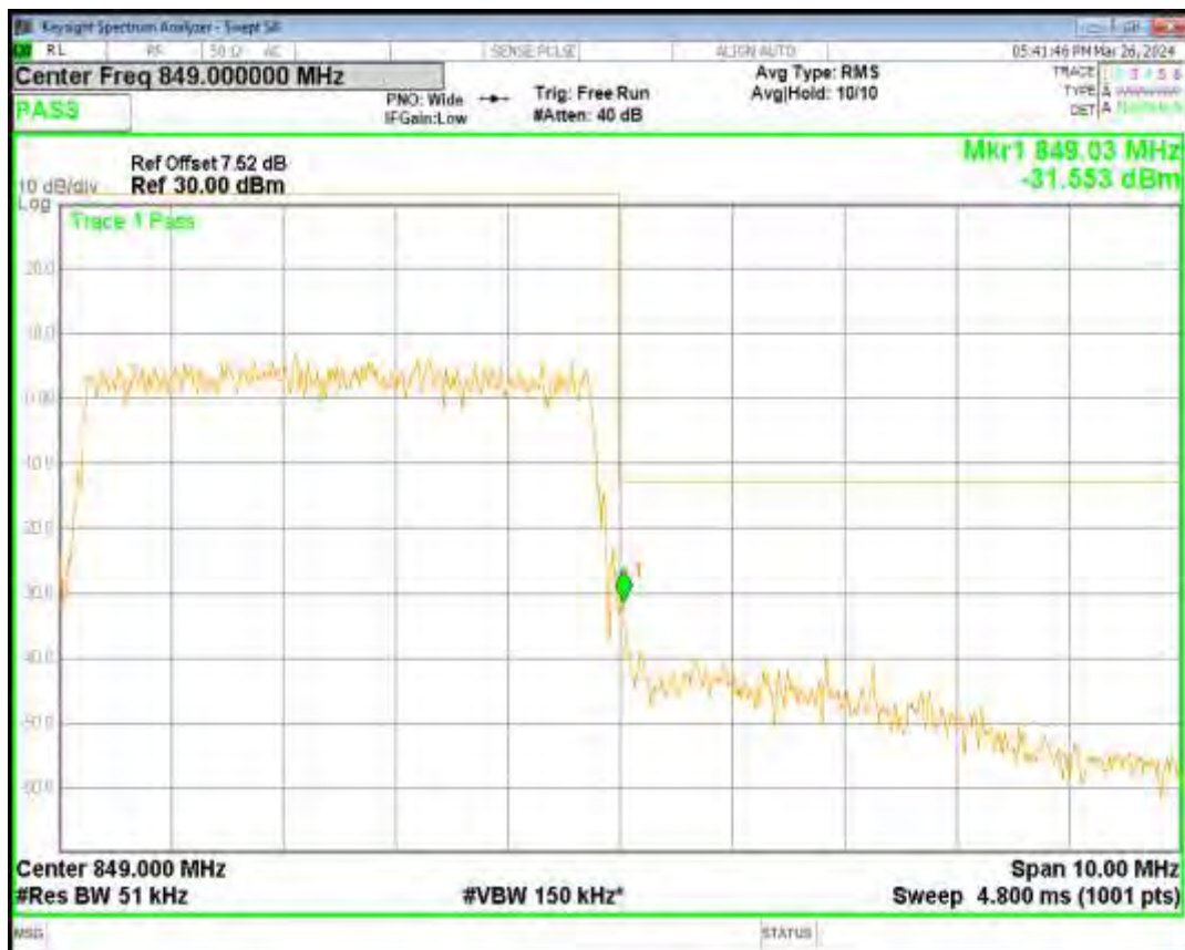
Band4 16QAM BW=1.4MHz Channel=19957 RB Size=6 Position=#0
