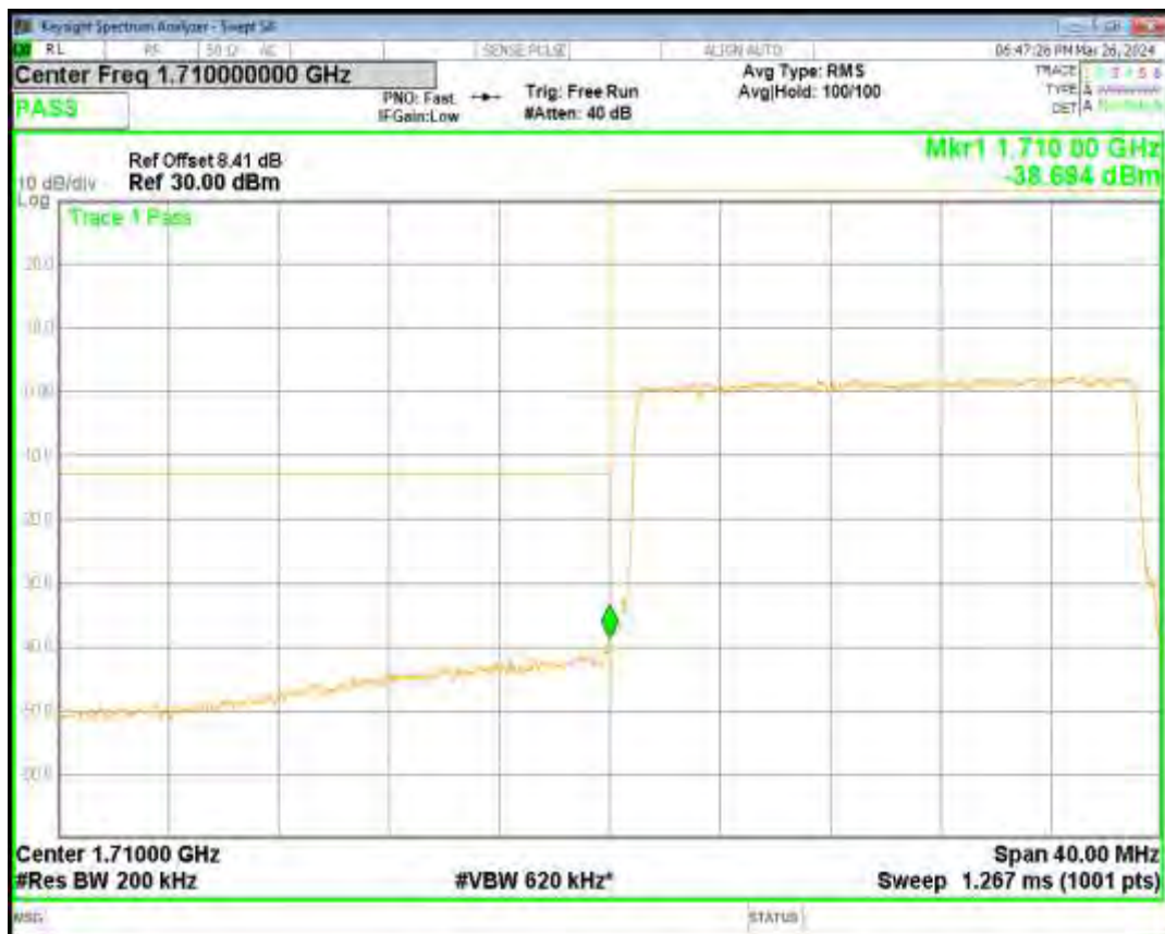
Band66 16QAM BW=15MHz Channel=132597 RB Size=75 Position=#0
