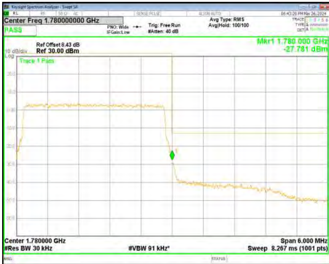
Band66 QPSK BW=5MHz Channel=132647 RB Size=25 Position=#0
