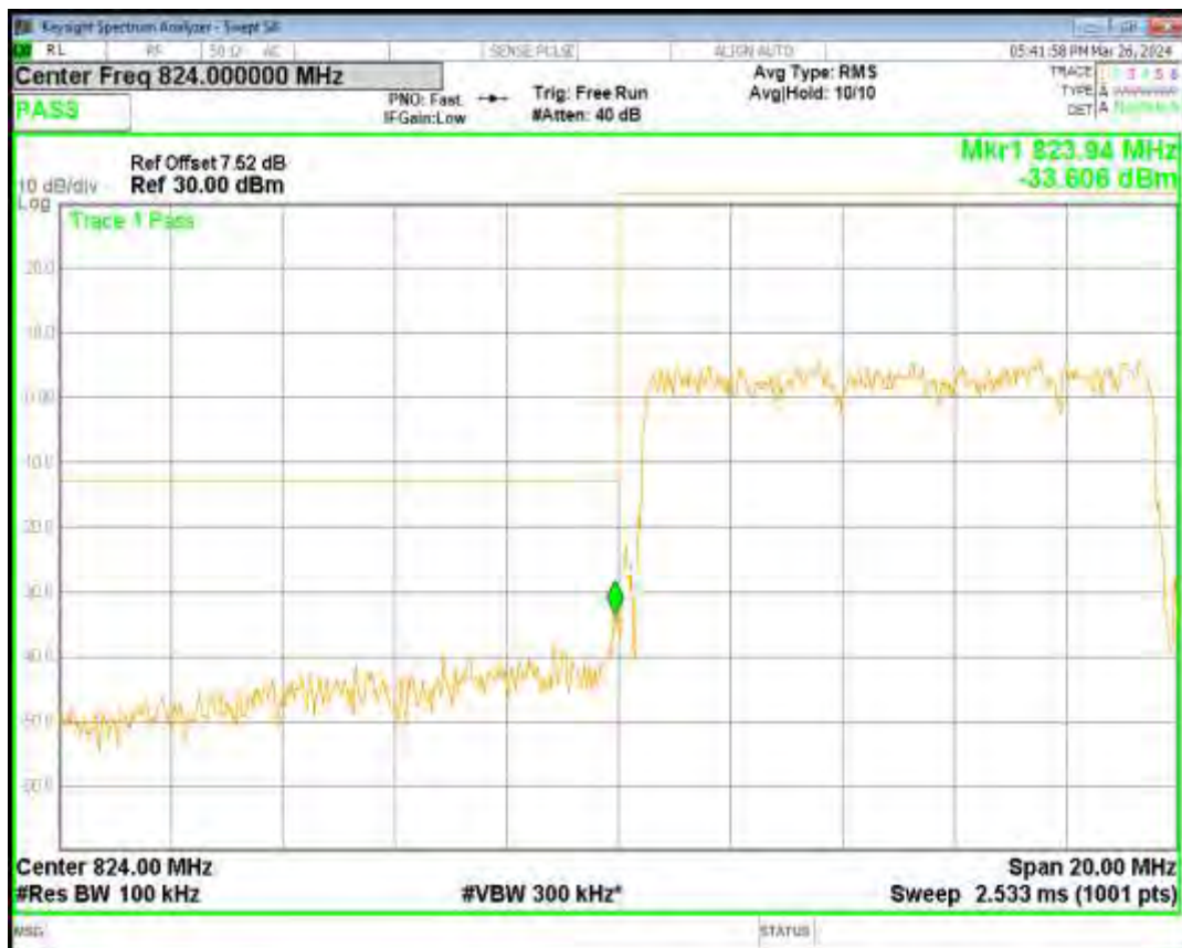
Band26(824-849) QPSK BW=10MHz Channel=26990 RB Size=50 Position=#0
