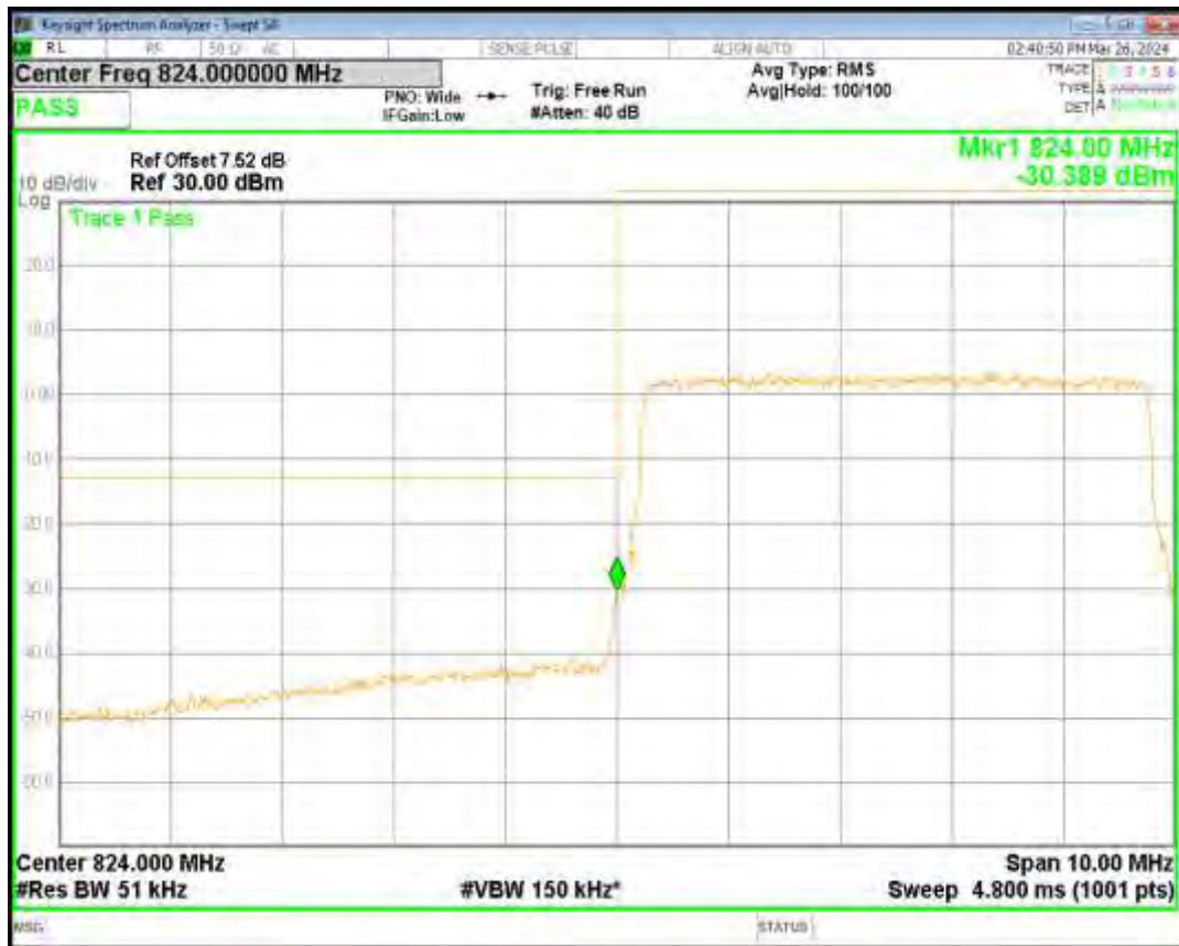
Band5 16QAM BW=5MHz Channel=20625 RB Size=25 Position=#0
