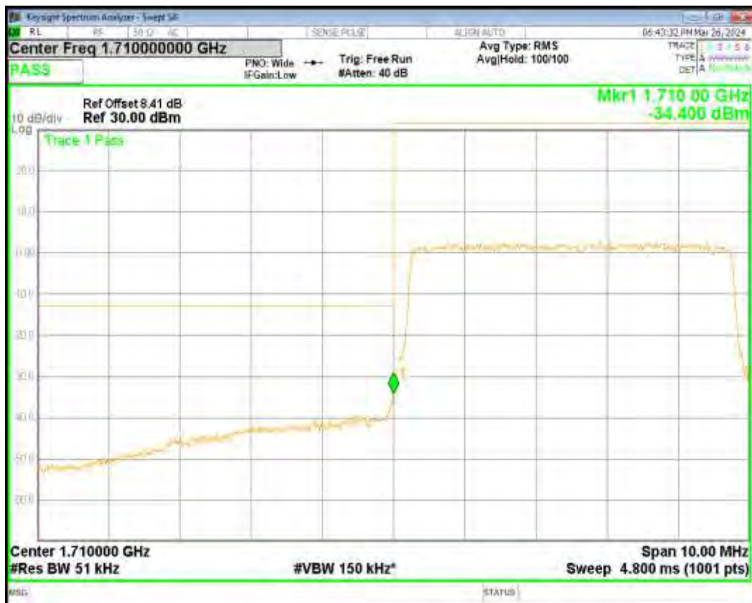
Band66 16QAM BW=3MHz Channel=132657 RB Size=15 Position=#0
