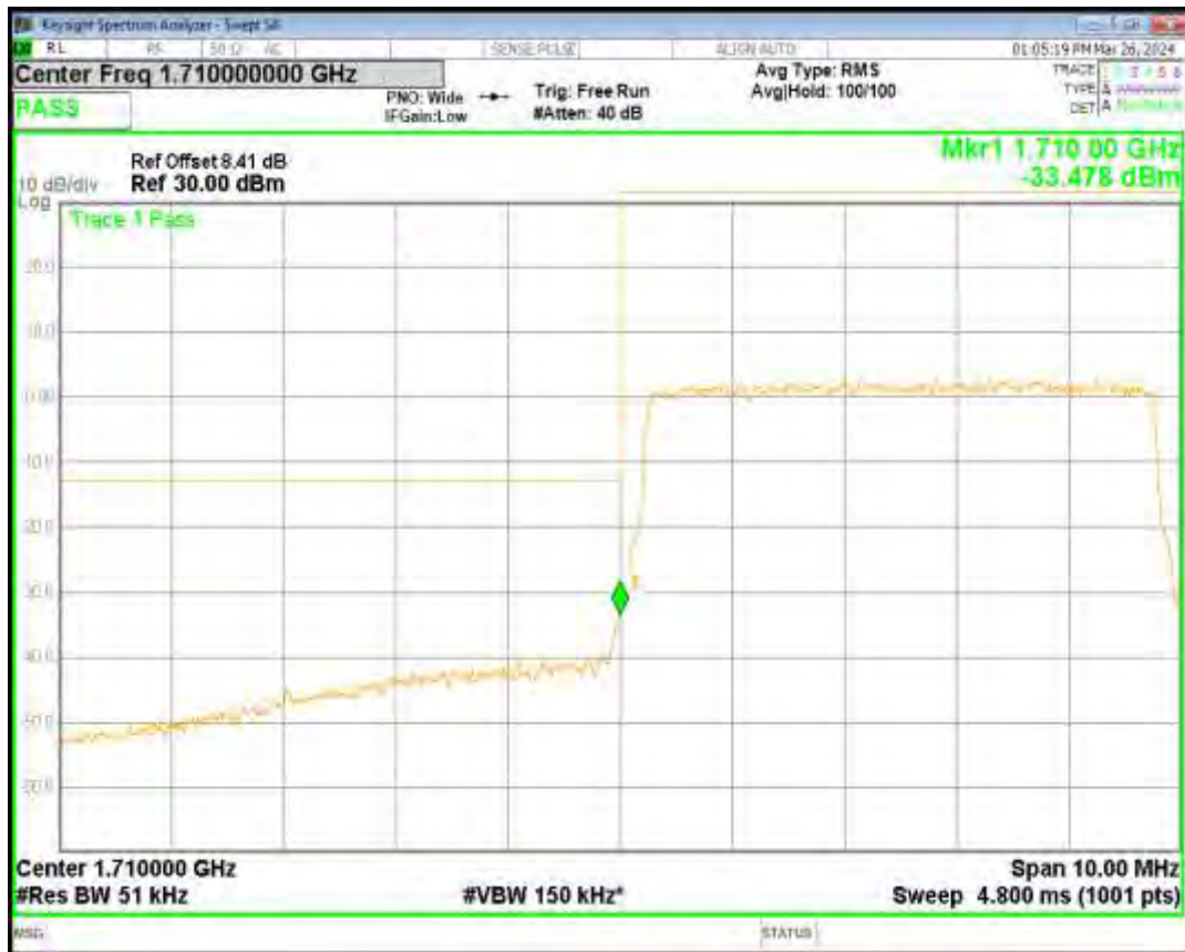
Band4 16QAM BW=3MHz Channel=20385 RB Size=15 Position=#0
