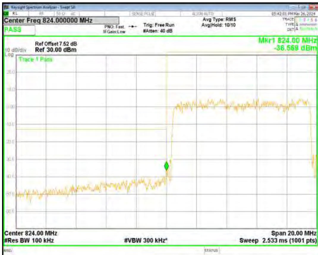
Band26(824-849) 16QAM BW=1.4MHz Channel=27033 RB Size=6 Position=#0
