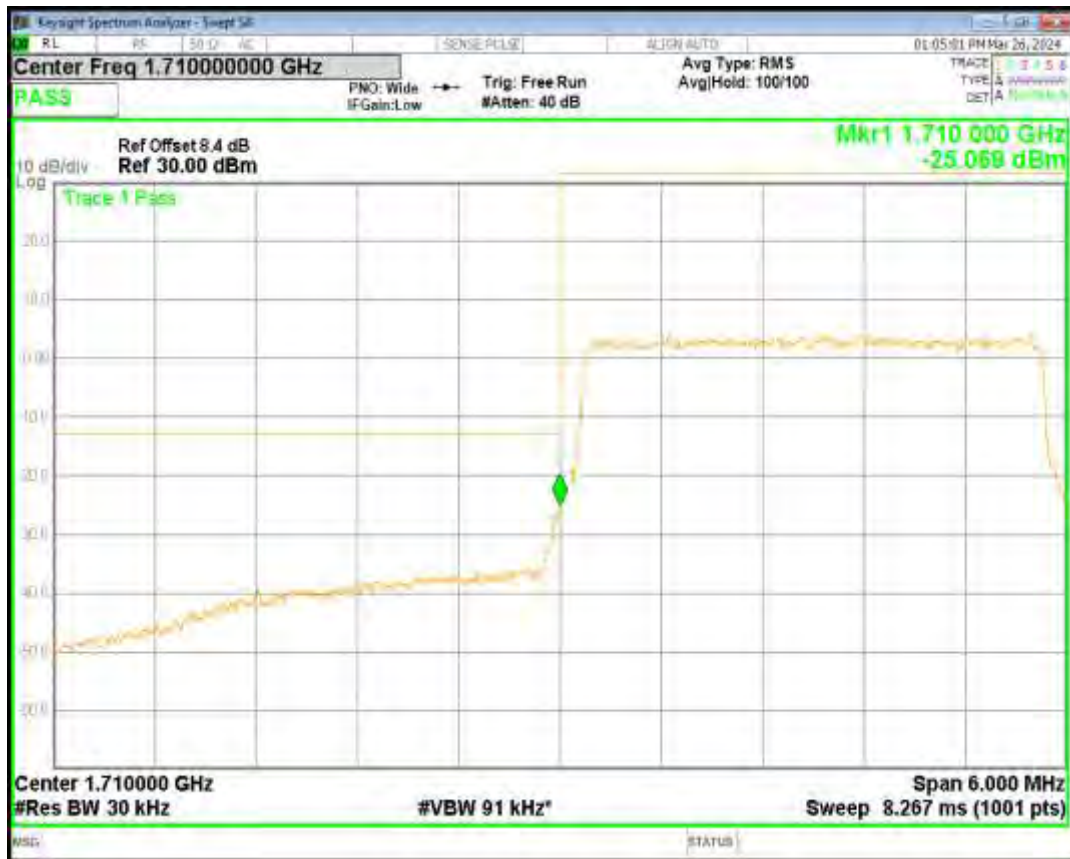
Band4 QPSK BW=3MHz Channel=20385 RB Size=15 Position=#0
