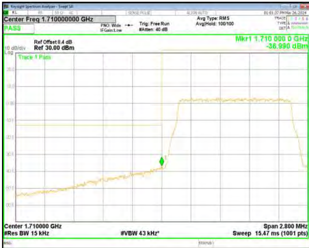
Band4 16QAM BW=1.4MHz Channel=20393 RB Size=6 Position=#0
