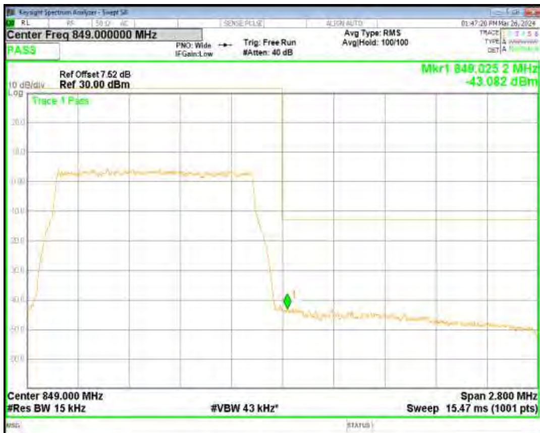
Band5 16QAM BW=10MHz Channel=20450 RB Size=50 Position=#0
