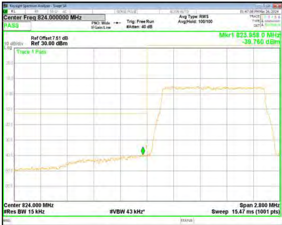
Band5 QPSK BW=1.4MHz Channel=20643 RB Size=6 Position=#0
