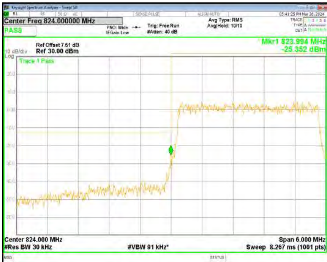
Band26(824-849) 16QAM BW=15MHz Channel=26965 RB Size=75 Position=#0
