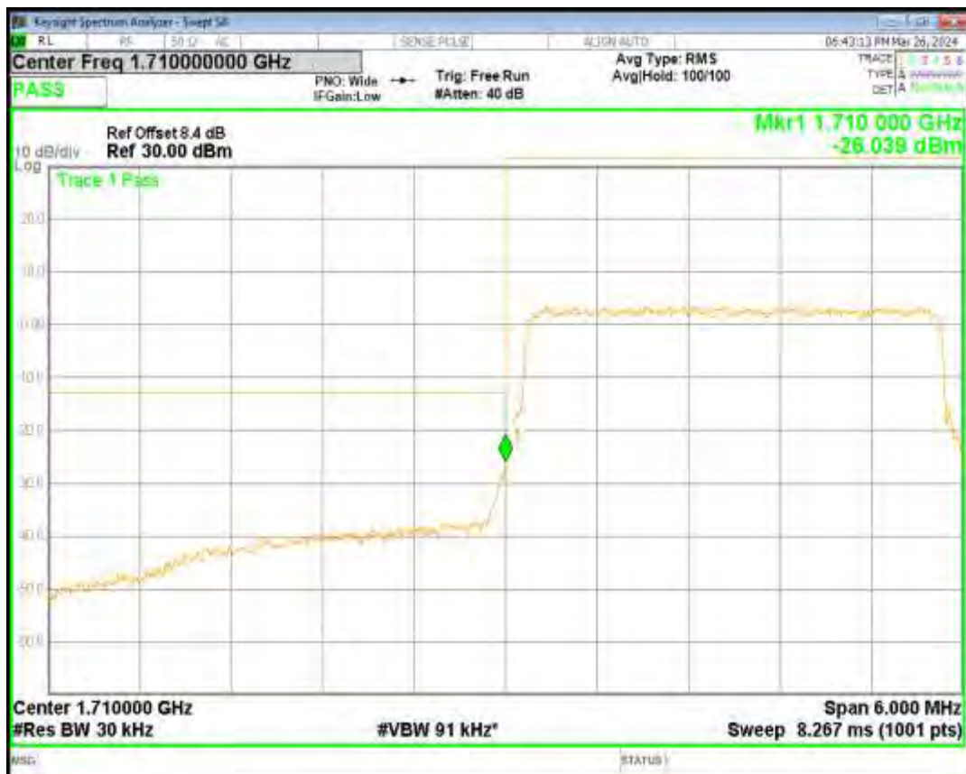
Band66 QPSK BW=3MHz Channel=132657 RB Size=15 Position=#0
