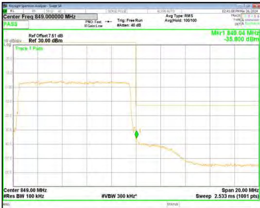
Band5 QPSK BW=3MHz Channel=20415 RB Size=15 Position=#0
