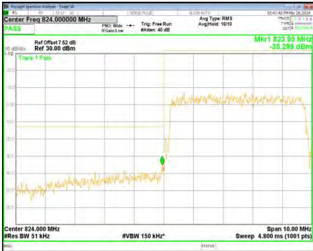
Band26(824-849) QPSK BW=1.4MHz Channel=26797 RB Size=6 Position=#0
