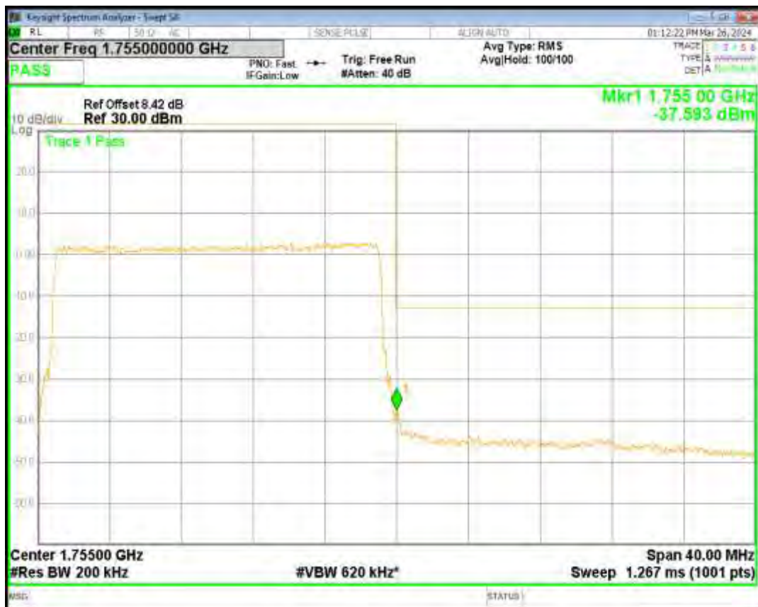
Band4 16QAM BW=20MHz Channel=20050 RB Size=100 Position=#0
