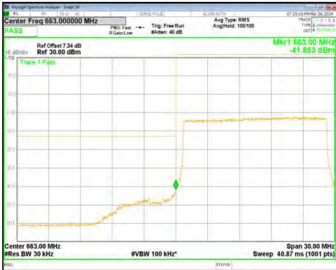
Band71 QPSK BW=15MHz Channel=133397 RB Size=75 Position=#0
