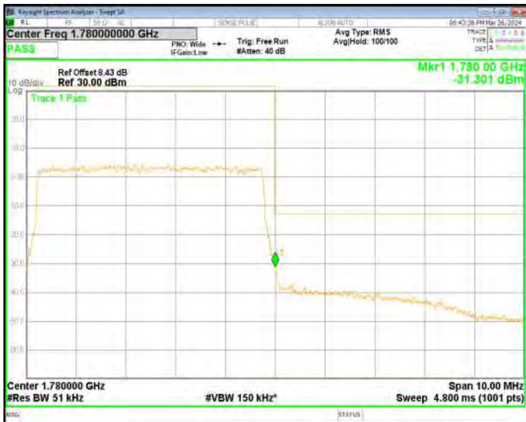
Band71 16QAM BW=10MHz Channel=133172 RB Size=50 Position=#0
