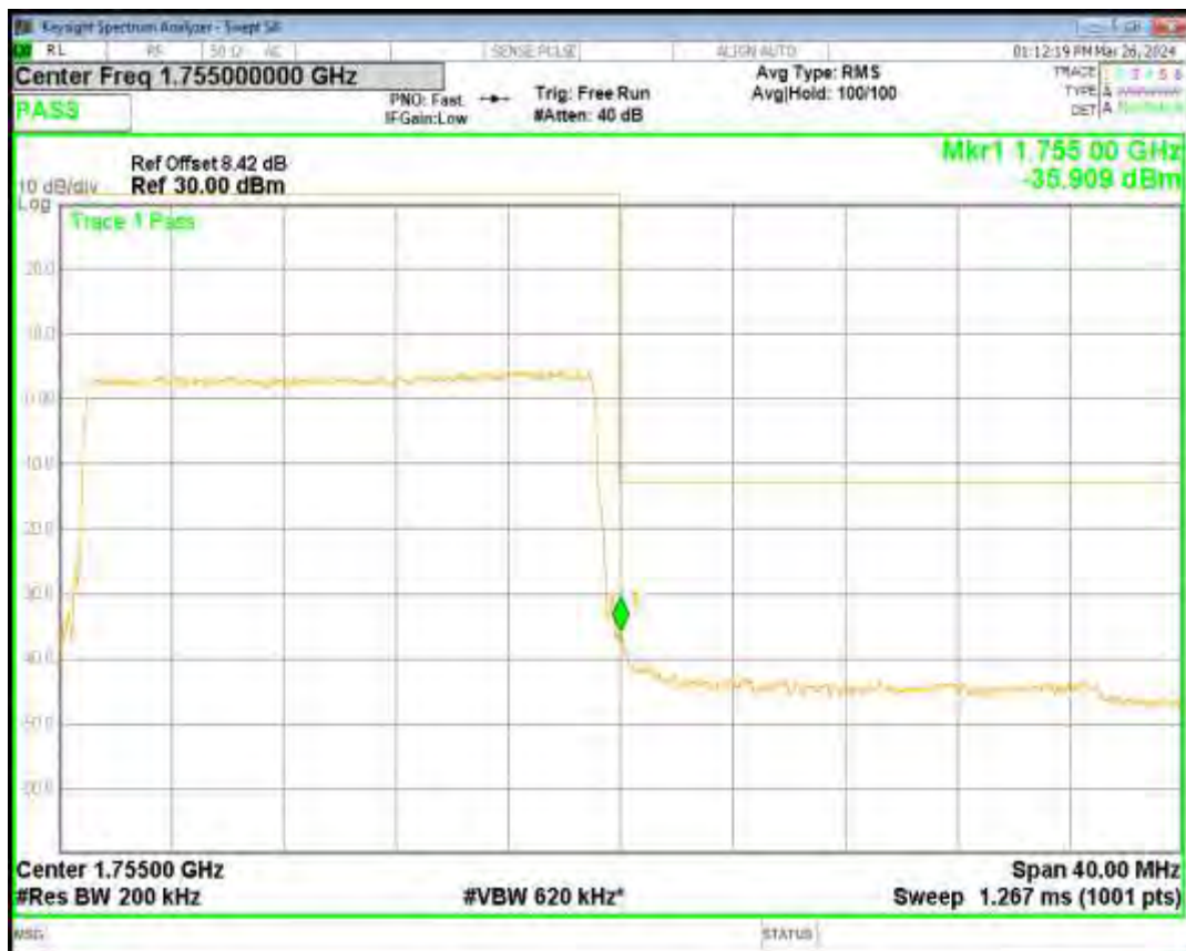
Band4 QPSK BW=3MHz Channel=19965 RB Size=15 Position=#0
