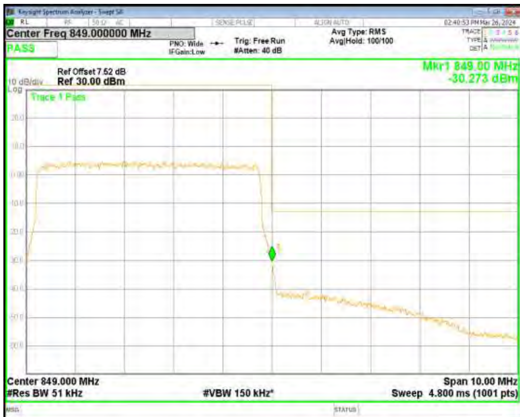
Band66 16QAM BW=1.4MHz Channel=131979 RB Size=6 Position=#0
