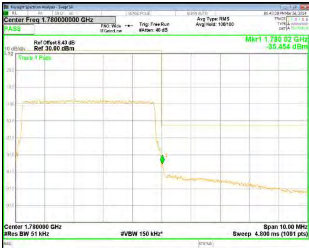
Band66 16QAM BW=20MHz Channel=132572 RB Size=100 Position=#0
