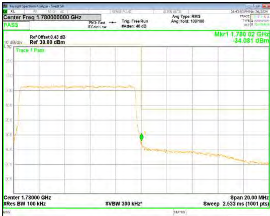
Band66 QPSK BW=10MHz Channel=132022 RB Size=50 Position=#0
