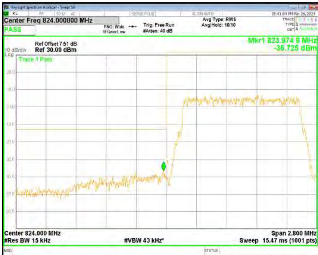
Band26(824-849) QPSK BW=1.4MHz Channel=27033 RB Size=6 Position=#0
