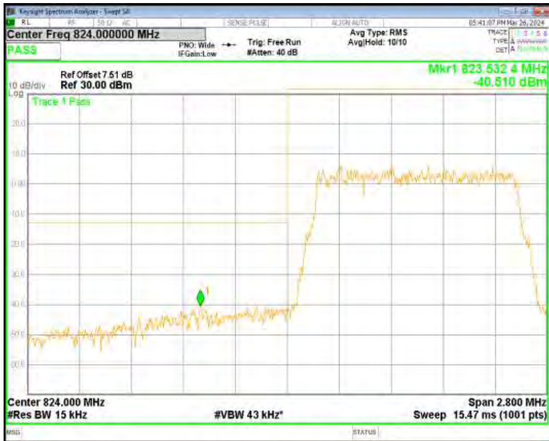
Band26(824-849) 16QAM BW=5MHz Channel=26815 RB Size=25 Position=#0
