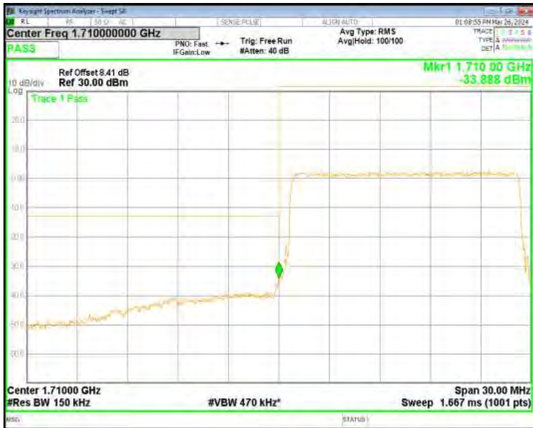
Band4 QPSK BW=1.4MHz Channel=19957 RB Size=6 Position=#0
