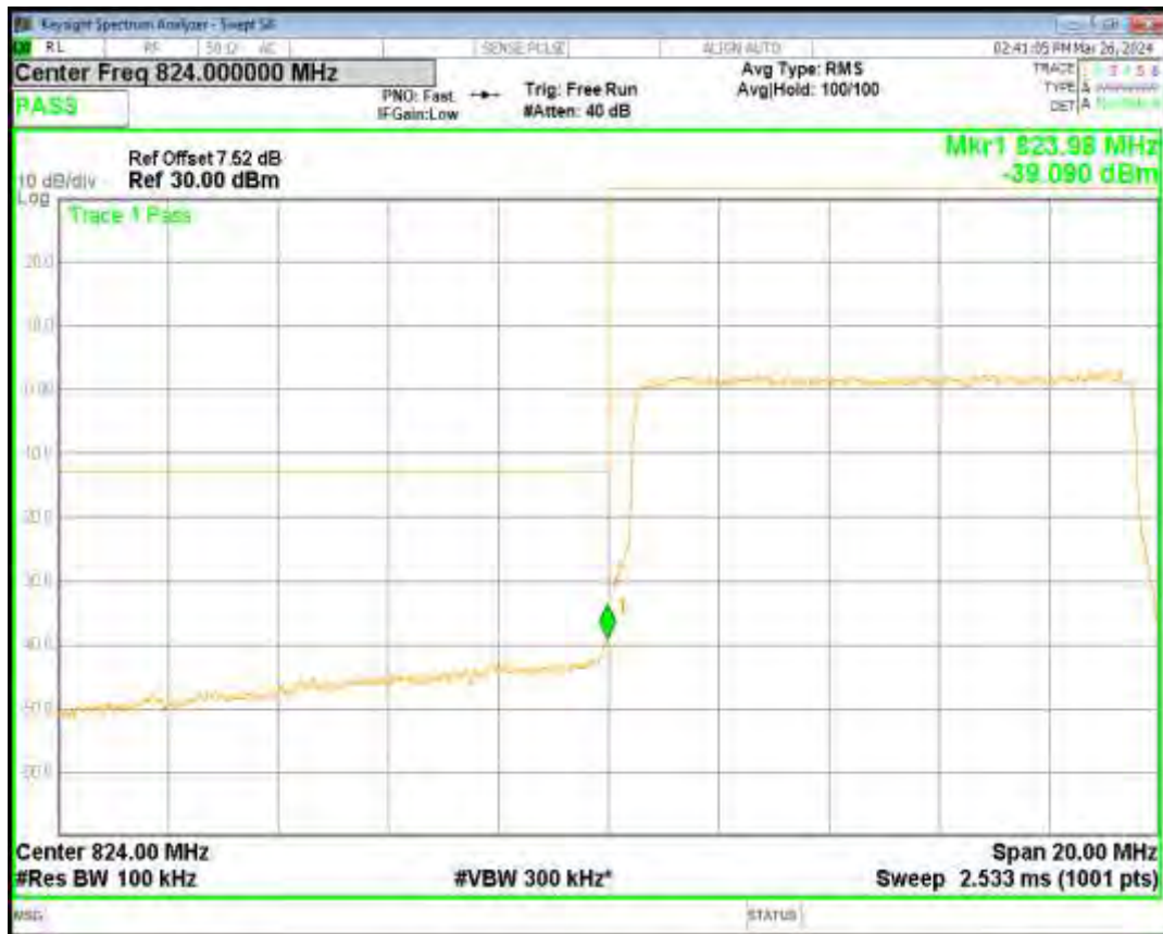
Band5 16QAM BW=10MHz Channel=20600 RB Size=50 Position=#0
