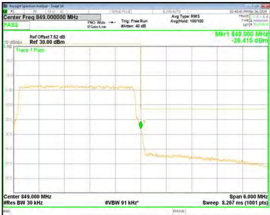
Band5 16QAM BW=5MHz Channel=20425 RB Size=25 Position=#0
