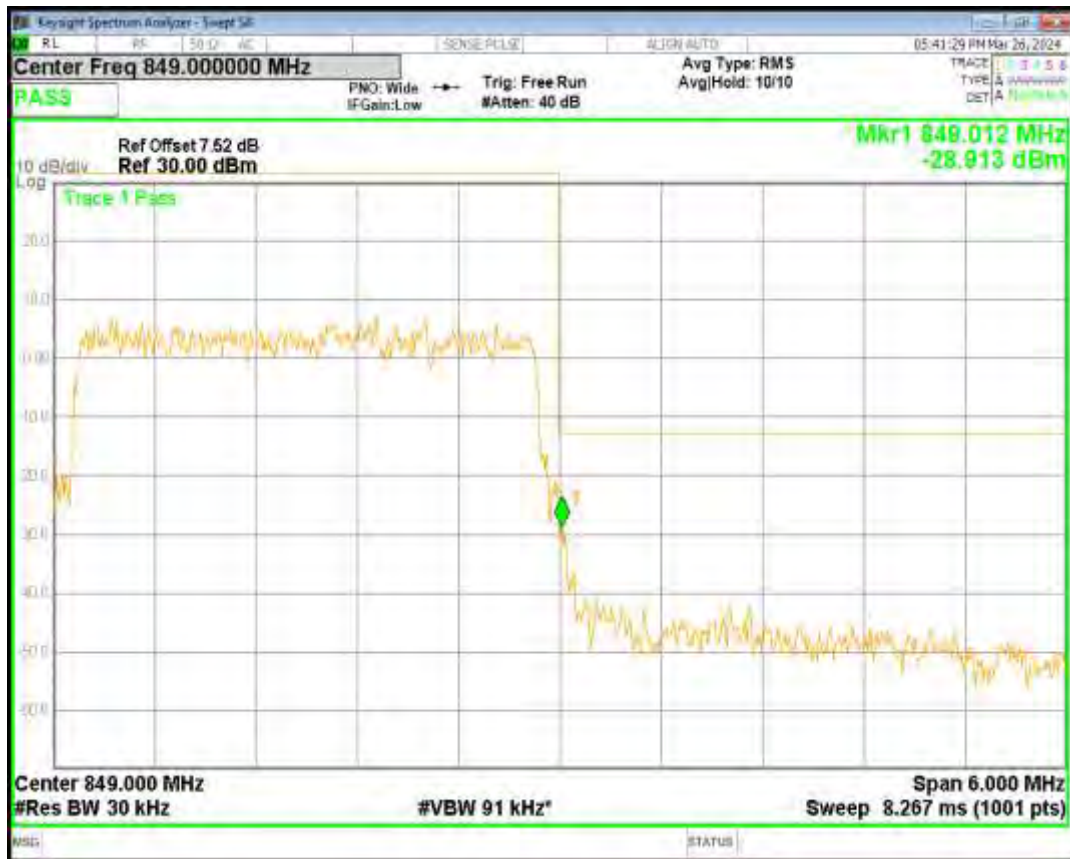
Band26(824-849) QPSK BW=5MHz Channel=27015 RB Size=25 Position=#0
