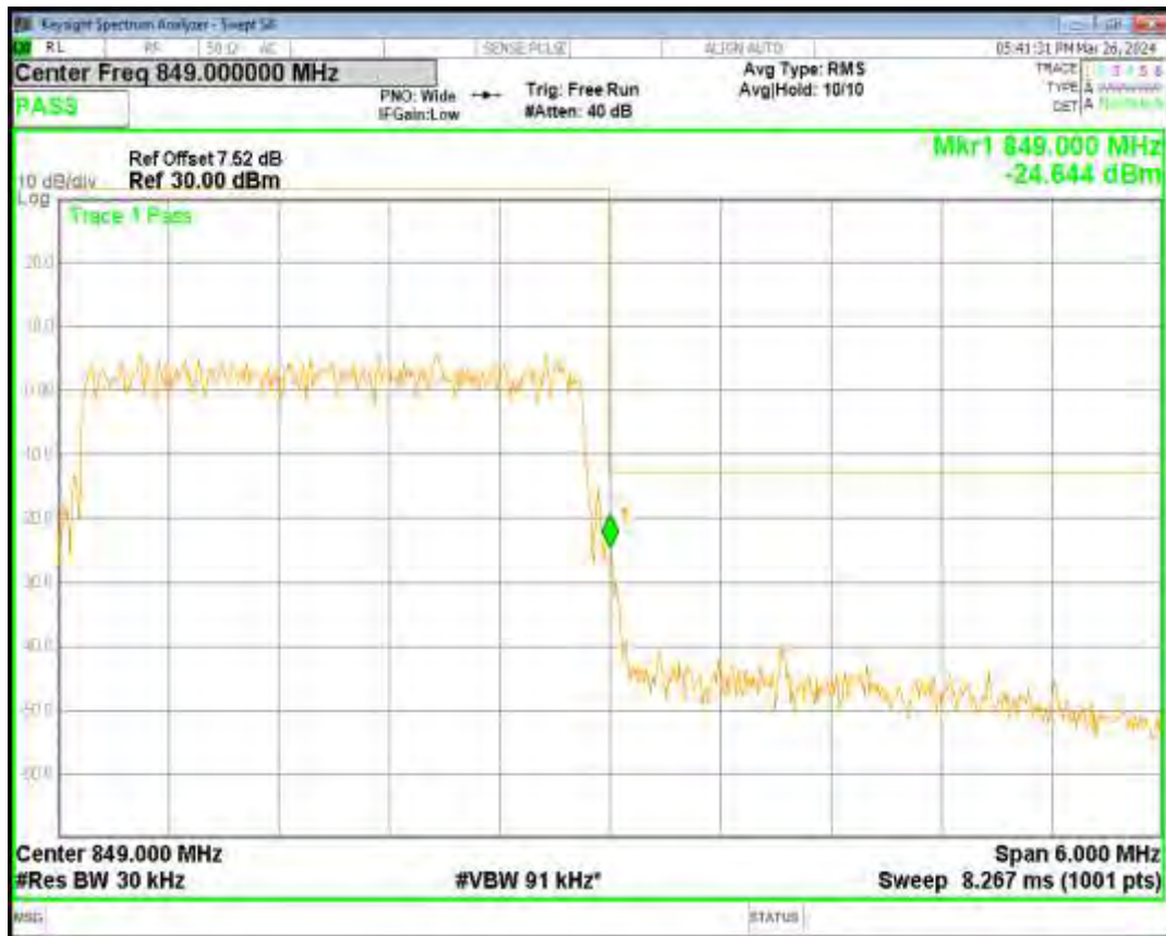
Band26(824-849) 16QAM BW=3MHz Channel=26805 RB Size=15 Position=#0
