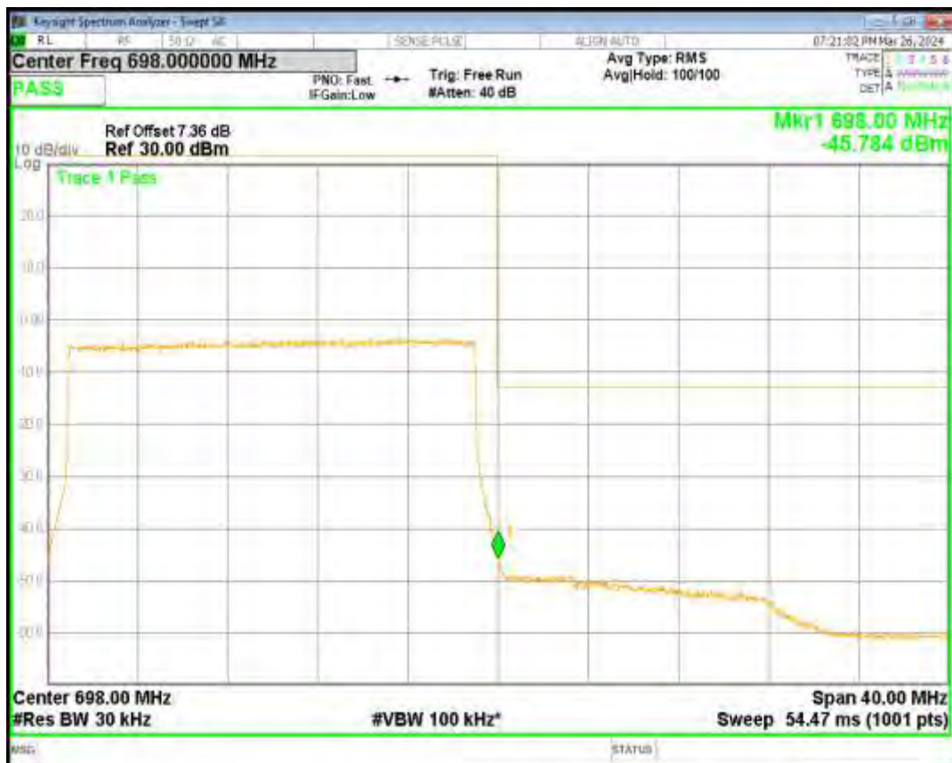
Band71 QPSK BW=5MHz Channel=133147 RB Size=25 Position=#0
