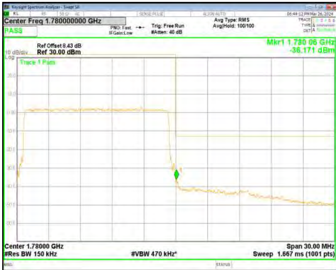
Band66 16QAM BW=15MHz Channel=132047 RB Size=75 Position=#0
