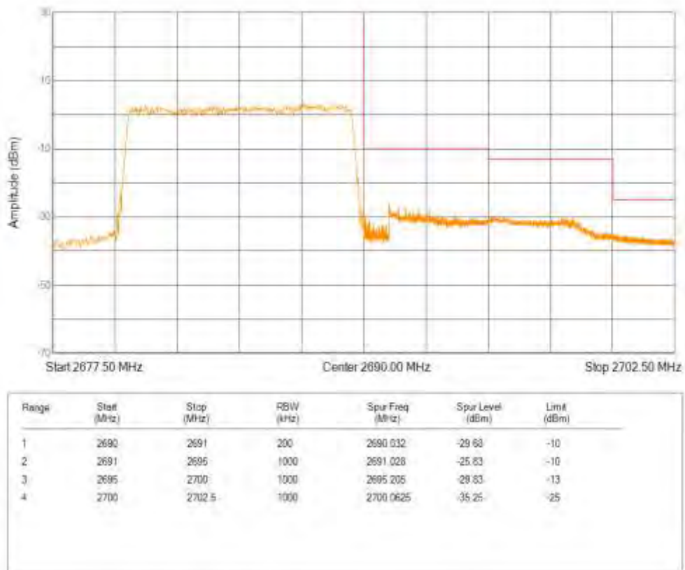
Band41 QPSK BW=15MHz Channel=39725 RB Size=75 Position=#0
