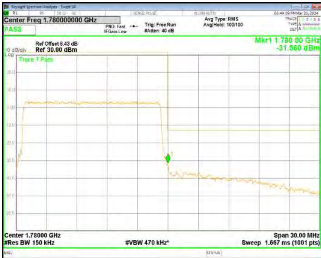
Band66 QPSK BW=20MHz Channel=132072 RB Size=100 Position=#0
