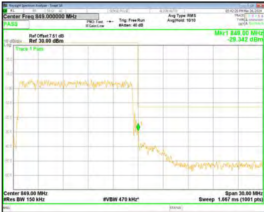
Band26(824-849) QPSK BW=3MHz Channel=26805 RB Size=15 Position=#0
