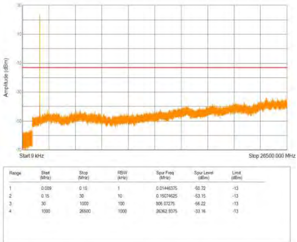
Band66 16QAM BW=10MHz Channel=132622 RB Size=50 Position=#0
