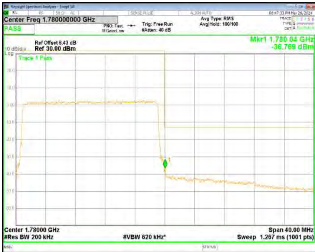
Band66 16QAM BW=20MHz Channel=132072 RB Size=100 Position=#0
