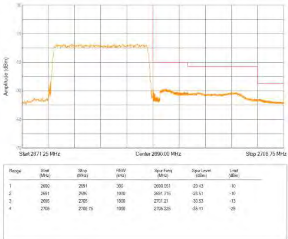
Band41 QPSK BW=20MHz Channel=39750 RB Size=100 Position=#0
