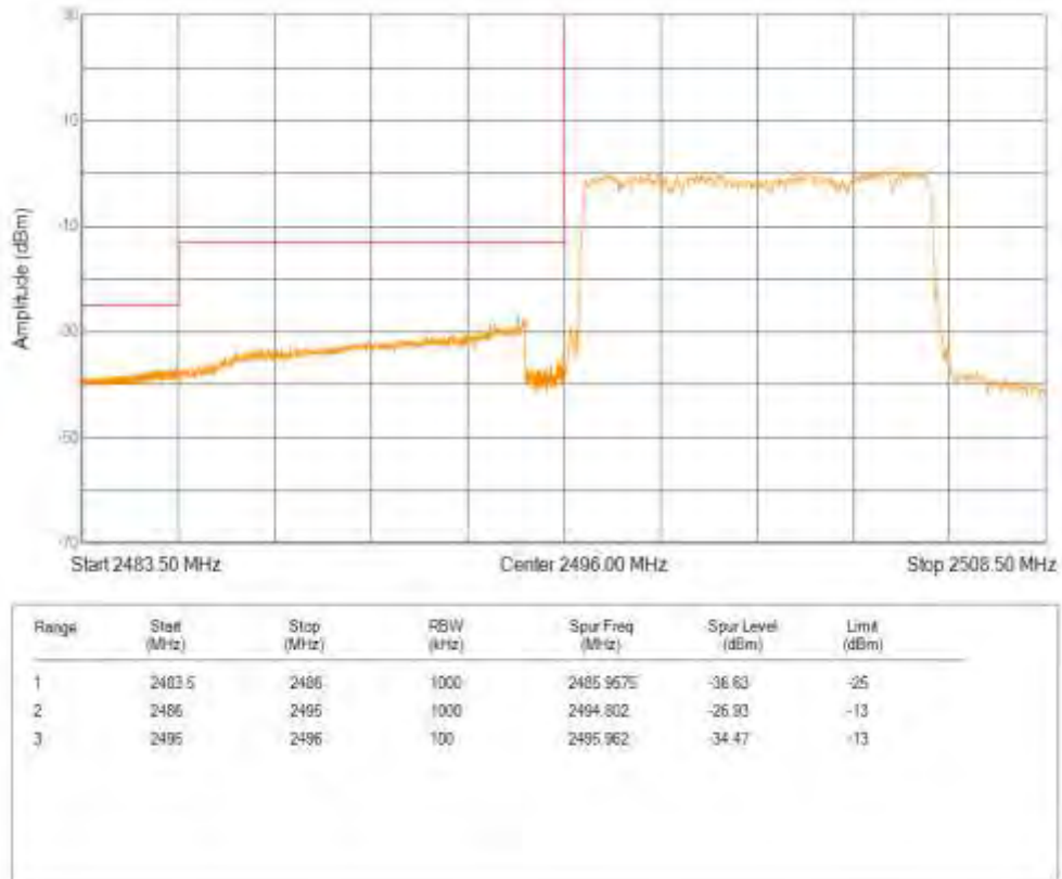
Band41 QPSK BW=10MHz Channel=41540 RB Size=50 Position=#0
