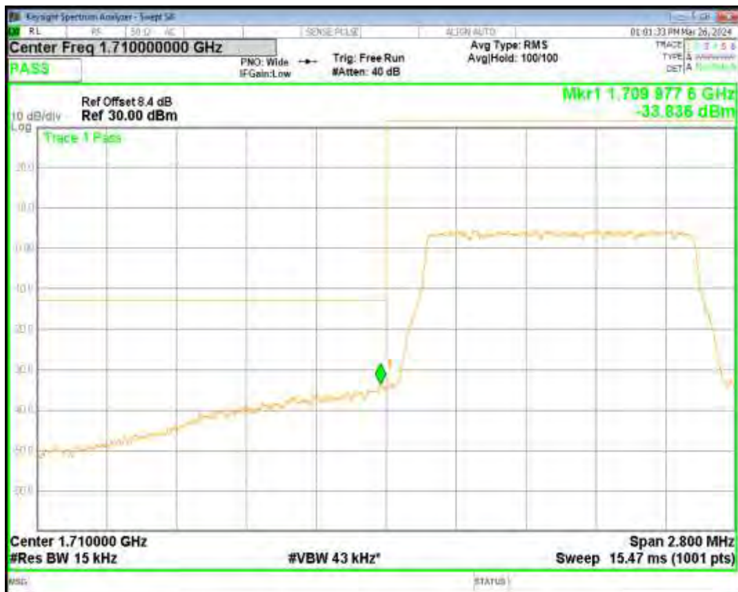
Band4 16QAM BW=5MHz Channel=19975 RB Size=25 Position=#0
