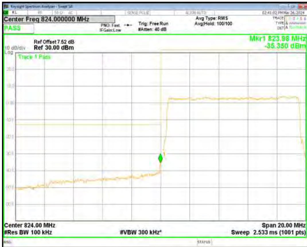
Band5 QPSK BW=10MHz Channel=20600 RB Size=50 Position=#0
