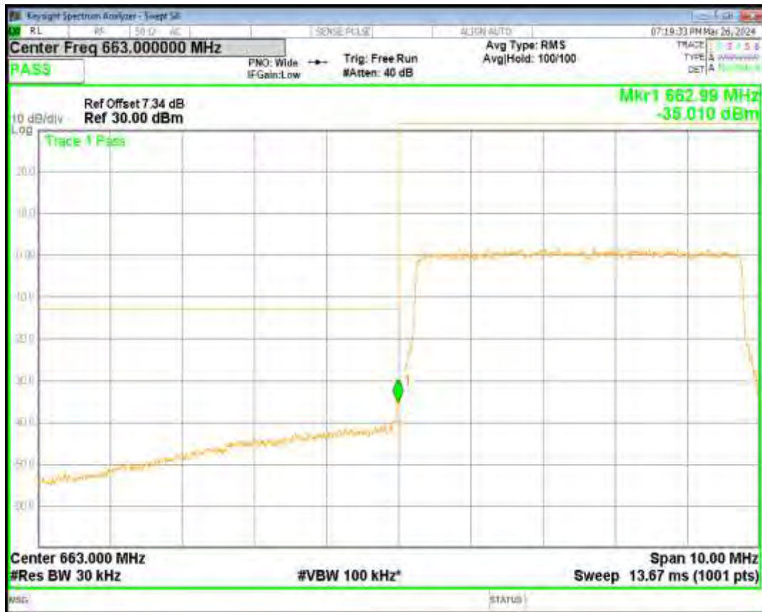
Band71 16QAM BW=5MHz Channel=133447 RB Size=25 Position=#0
