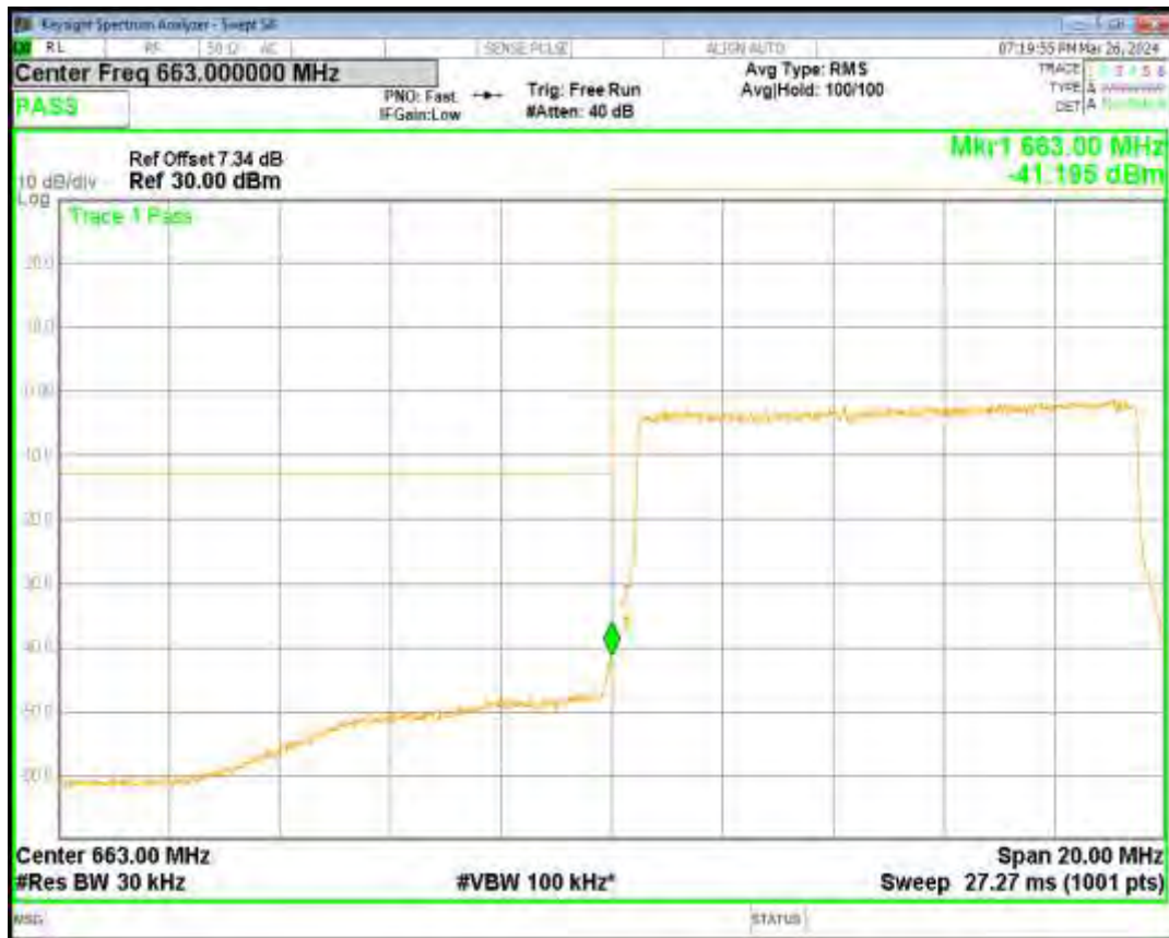
Band71 16QAM BW=10MHz Channel=133422 RB Size=50 Position=#0
