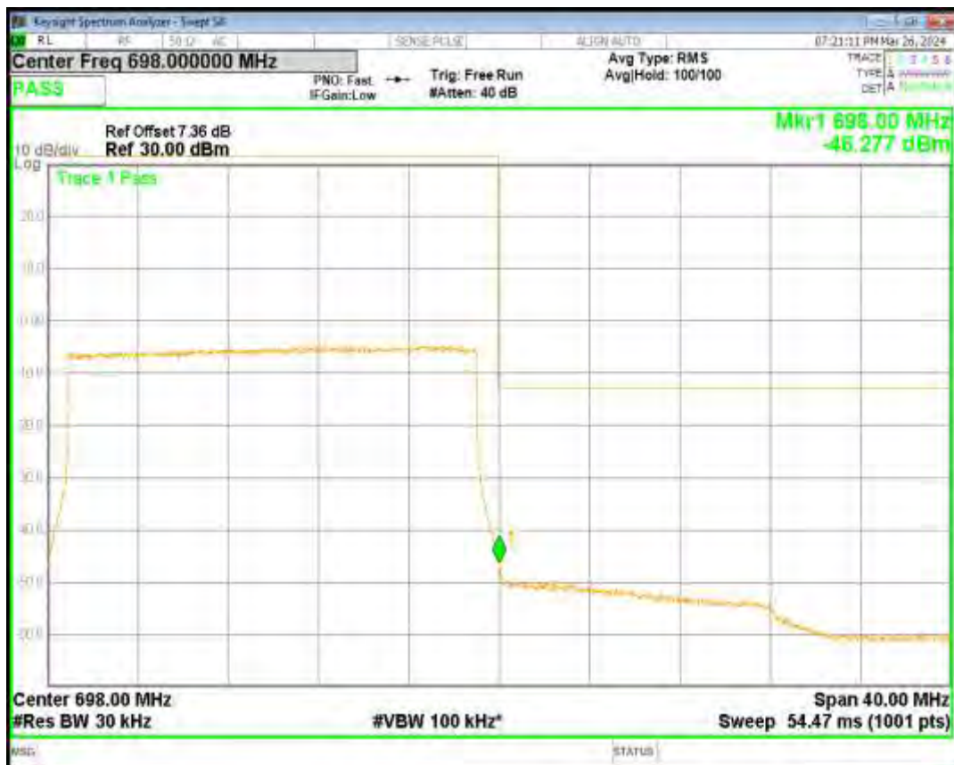
Band71 16QAM BW=5MHz Channel=133147 RB Size=25 Position=#0
