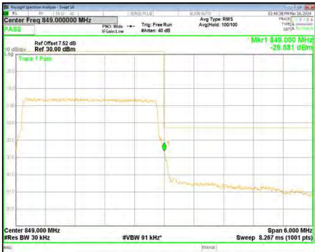
Band5 QPSK BW=5MHz Channel=20425 RB Size=25 Position=#0
