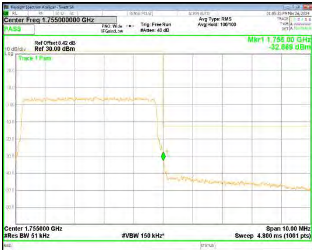
Band41 16QAM BW=10MHz Channel=39700 RB Size=50 Position=#0
