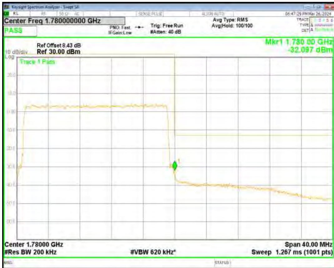
Band66 QPSK BW=3MHz Channel=131987 RB Size=15 Position=#0
