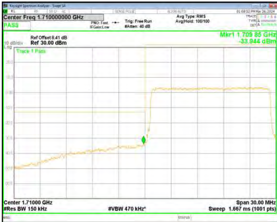
Band4 QPSK BW=15MHz Channel=20325 RB Size=75 Position=#0
