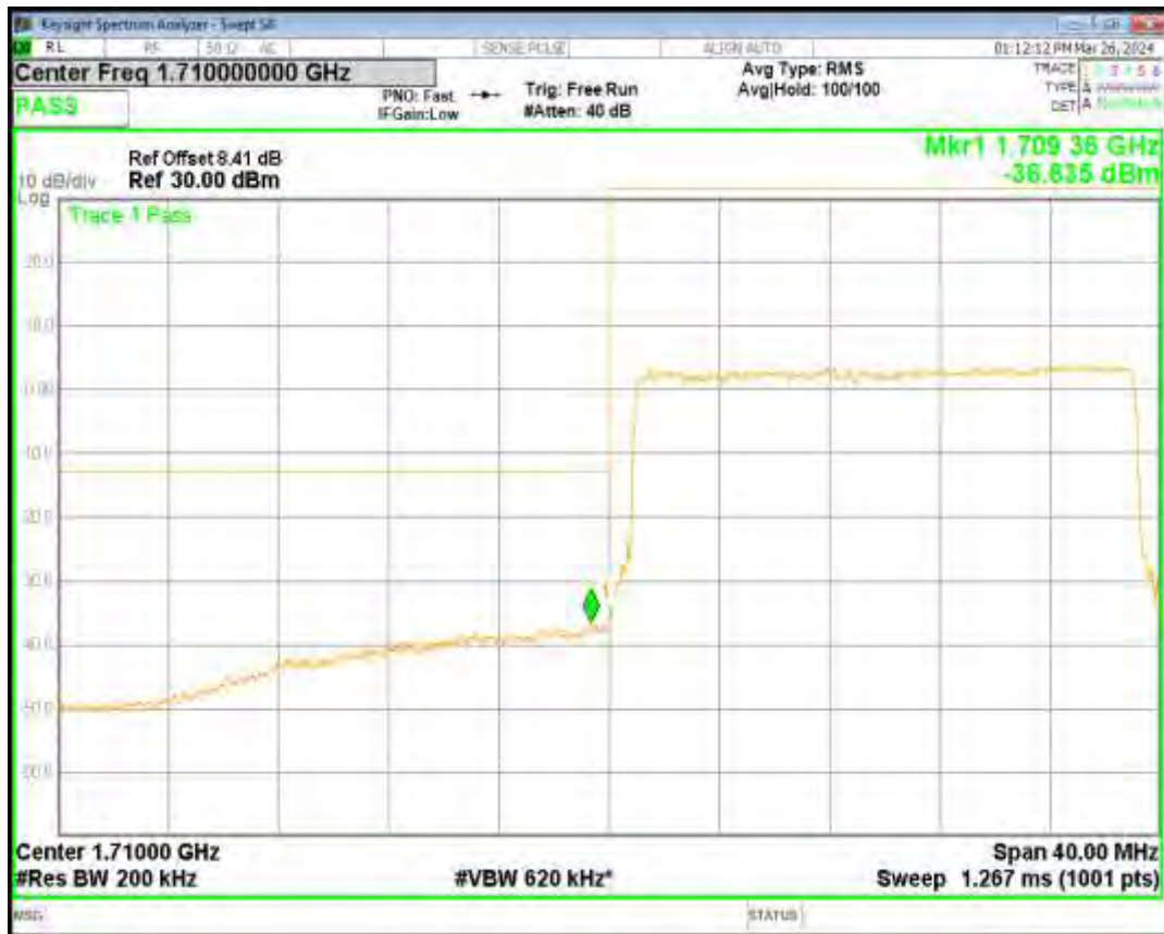
Band4 QPSK BW=20MHz Channel=20300 RB Size=100 Position=#0
