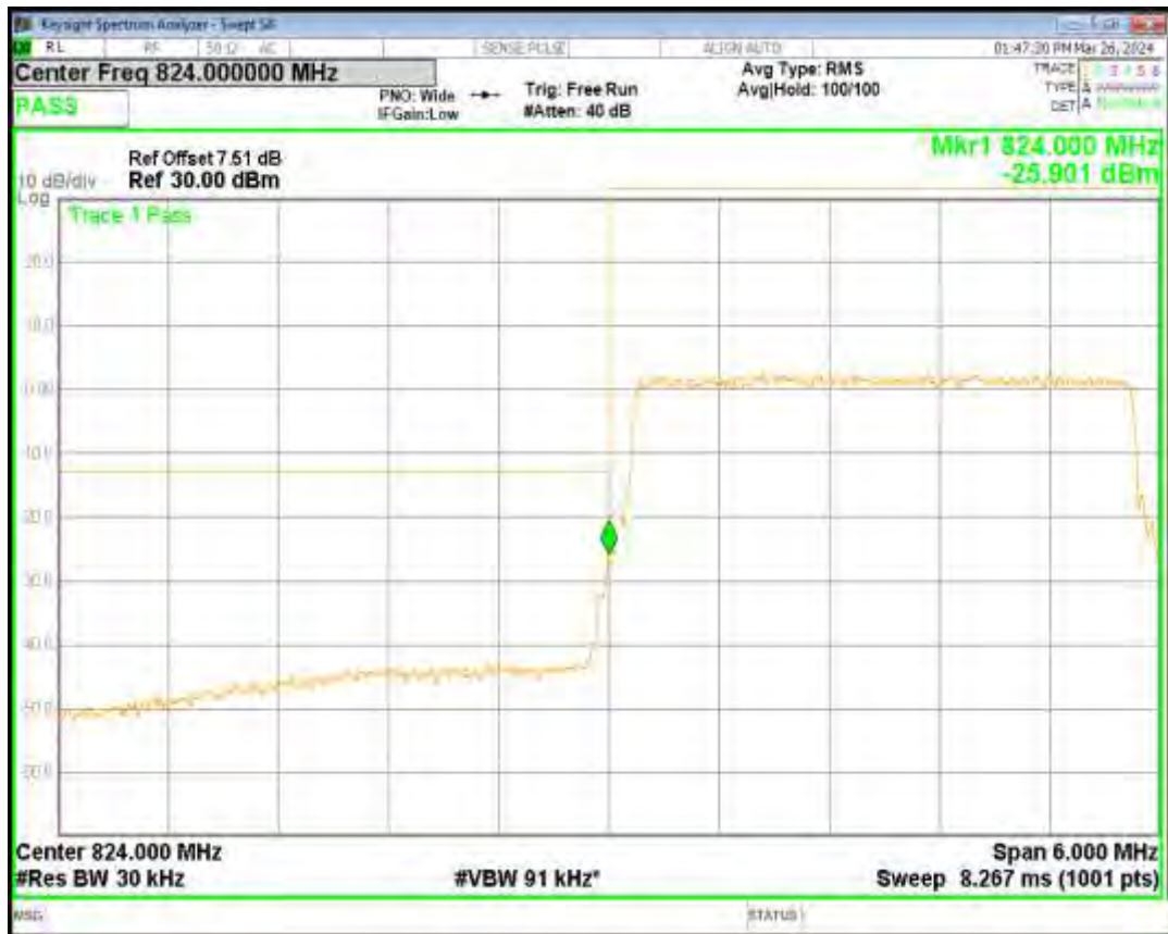
Band5 16QAM BW=3MHz Channel=20635 RB Size=15 Position=#0
