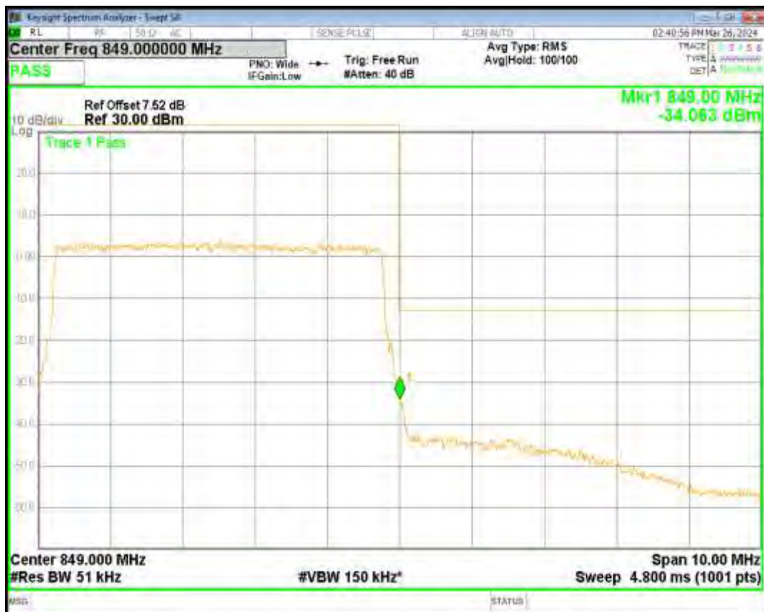
Band5 QPSK BW=1.4MHz Channel=20407 RB Size=6 Position=#0
