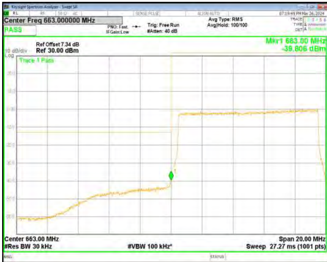
Band71 QPSK BW=10MHz Channel=133422 RB Size=50 Position=#0
