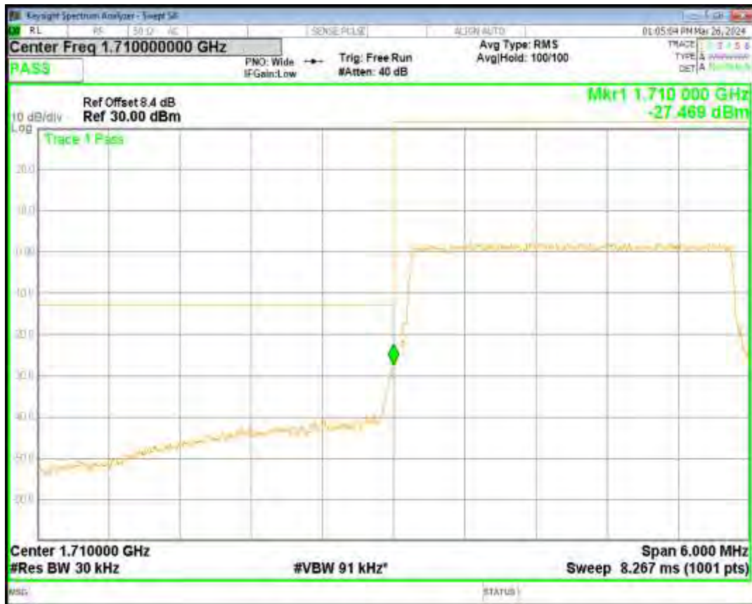
Band4 QPSK BW=1.4MHz Channel=20393 RB Size=6 Position=#0
