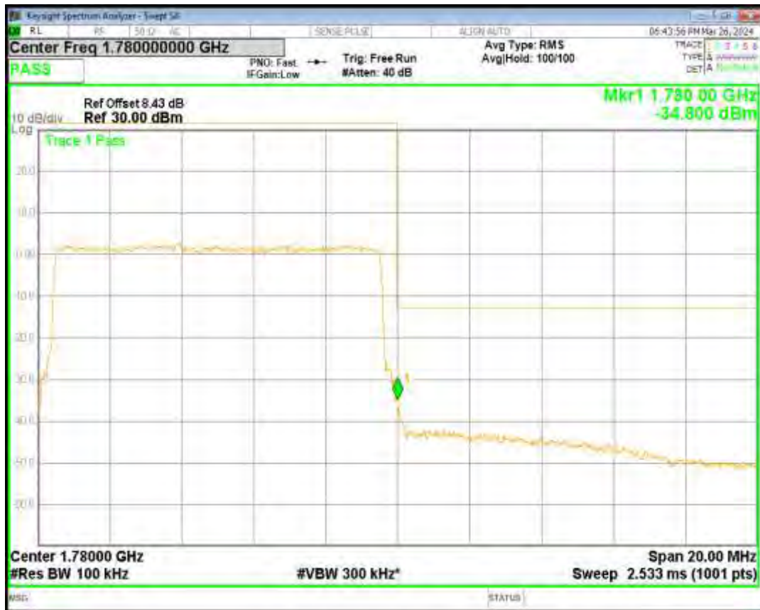
Band66 16QAM BW=3MHz Channel=131987 RB Size=15 Position=#0
