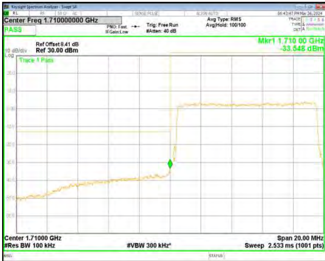
Band66 QPSK BW=1.4MHz Channel=132665 RB Size=6 Position=#0
