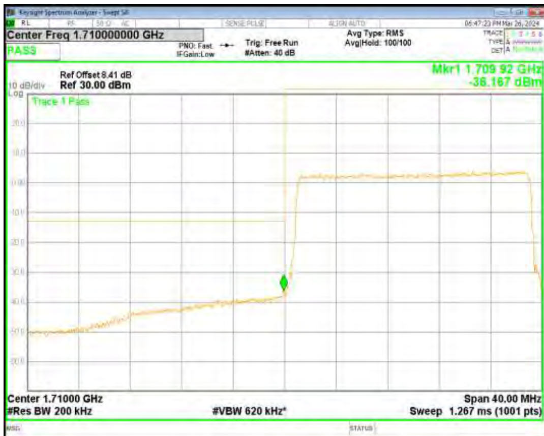
Band66 QPSK BW=20MHz Channel=132572 RB Size=100 Position=#0
