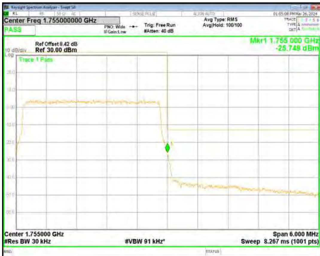
Band4 QPSK BW=5MHz Channel=19975 RB Size=25 Position=#0
