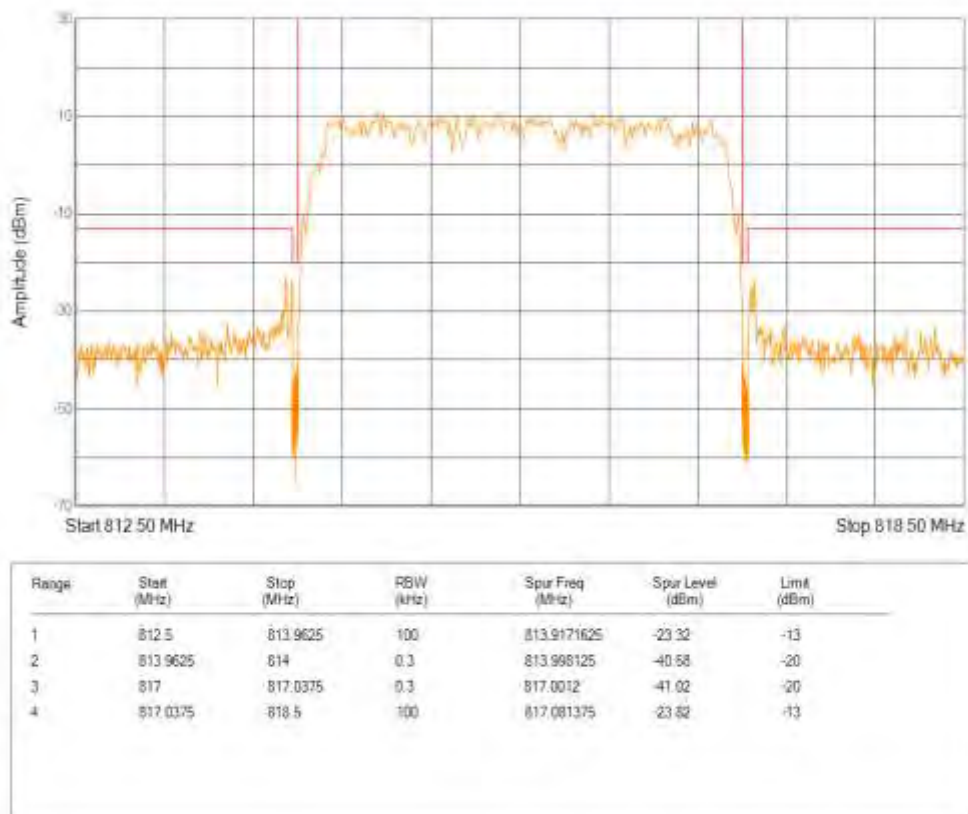
Band26(814-824) QPSK BW=3MHz Channel=26775 RB Size=15 Position=#0
