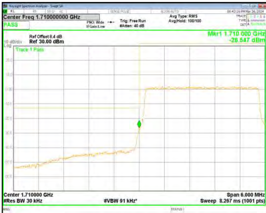
Band66 QPSK BW=5MHz Channel=131997 RB Size=25 Position=#0
