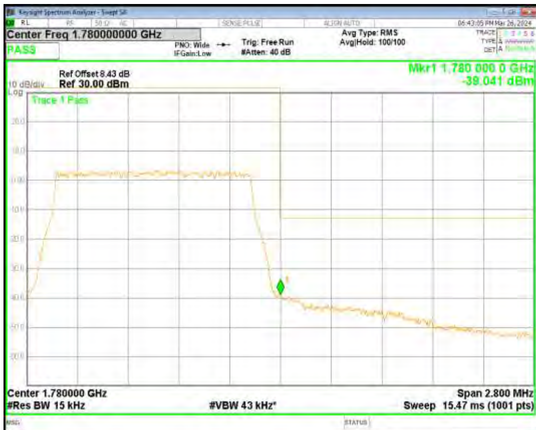
Band66 16QAM BW=10MHz Channel=132022 RB Size=50 Position=#0
