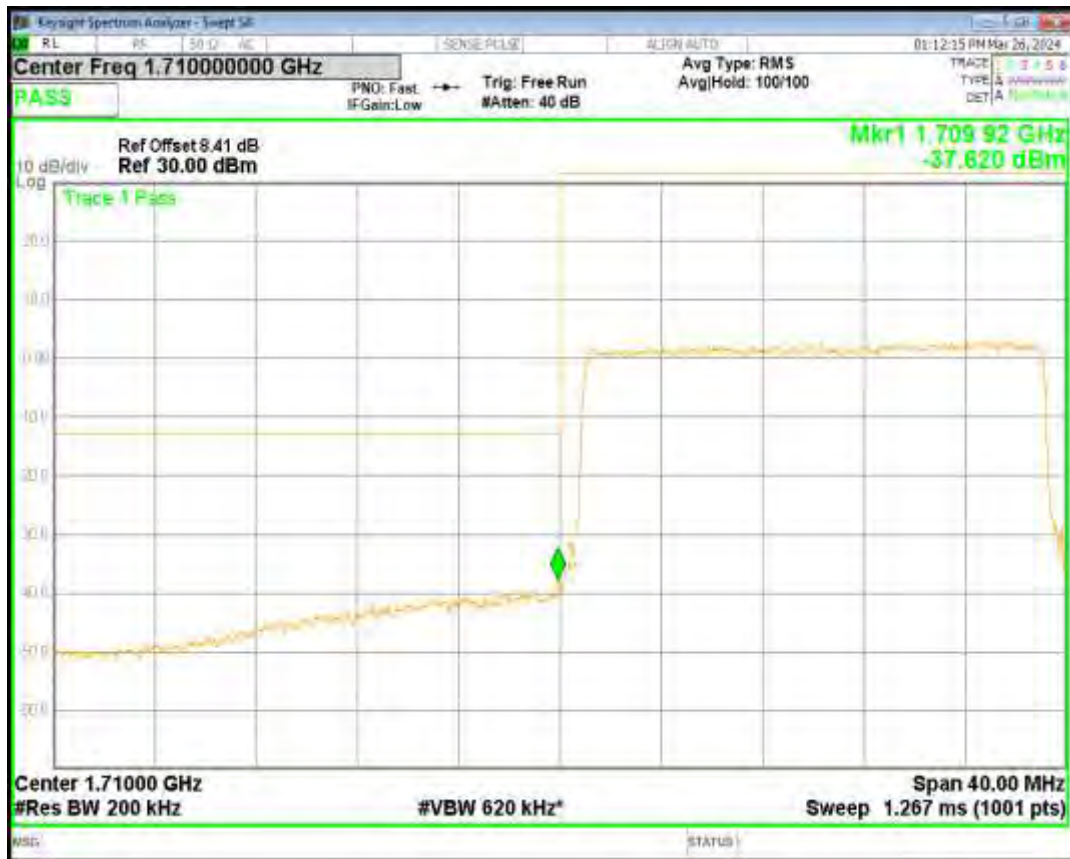
Band4 16QAM BW=15MHz Channel=20325 RB Size=75 Position=#0
