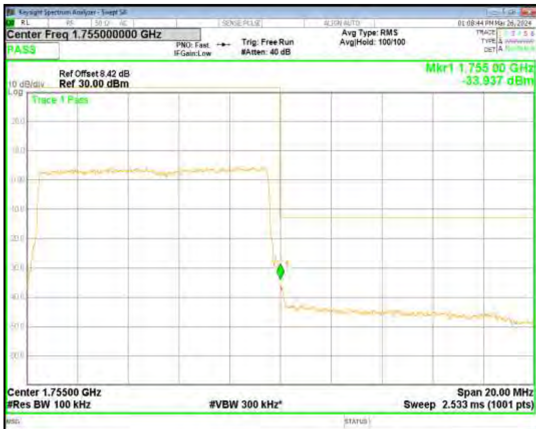
Band4 QPSK BW=15MHz Channel=20025 RB Size=75 Position=#0
