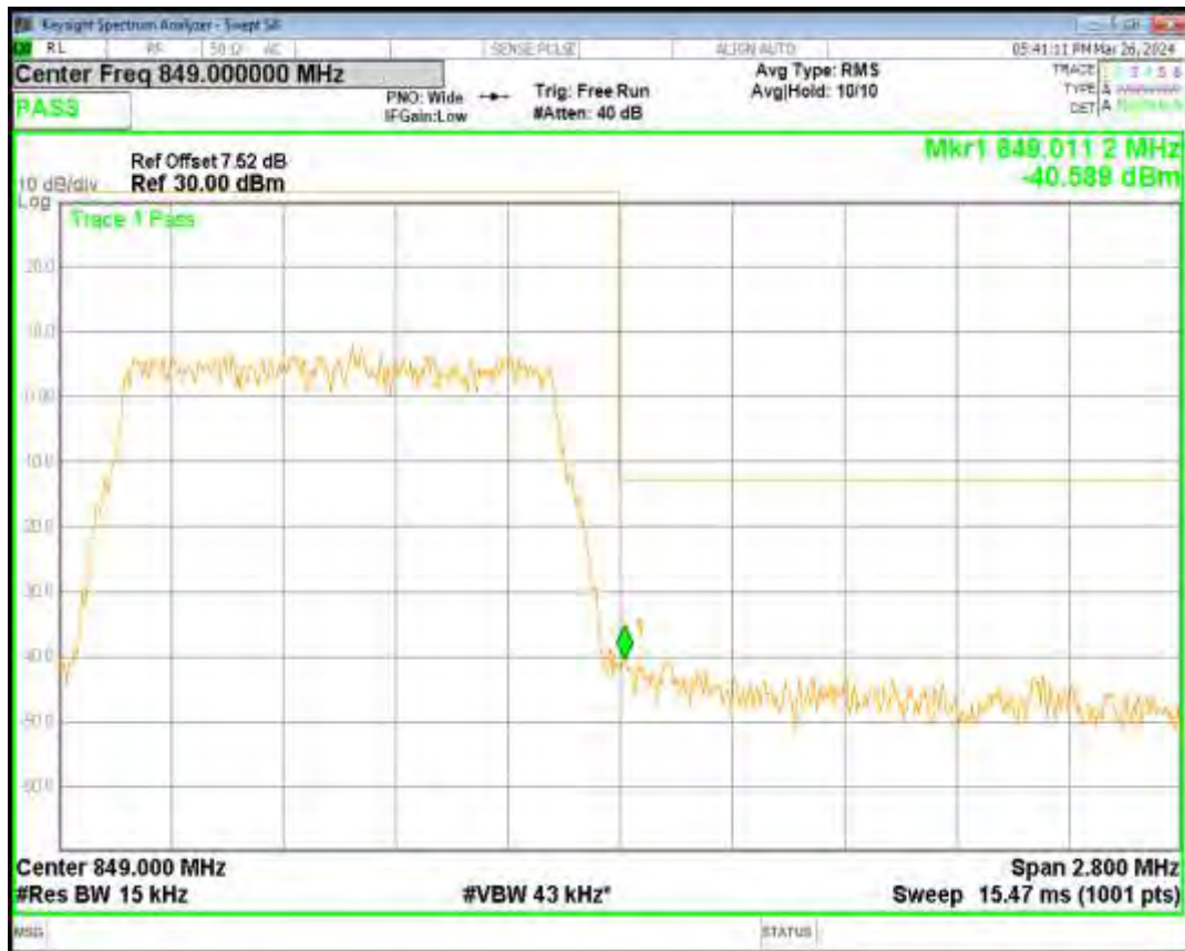
Band26(824-849) QPSK BW=10MHz Channel=26840 RB Size=50 Position=#0
