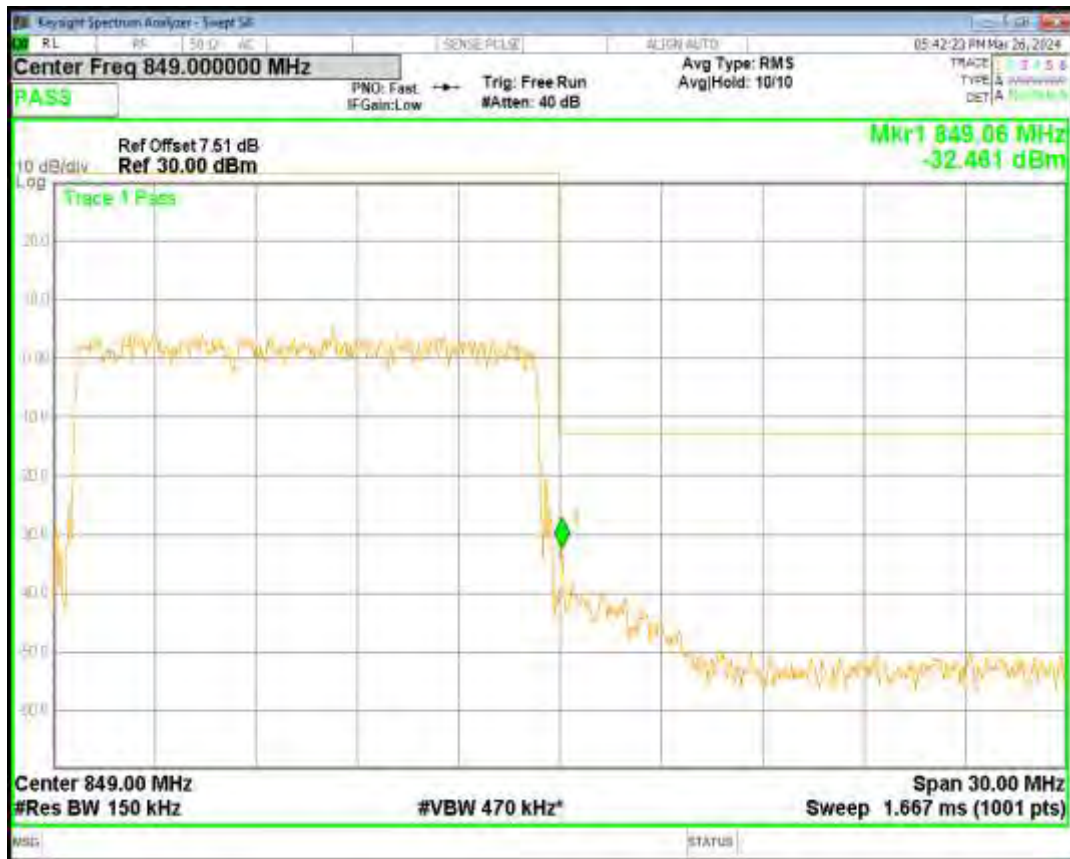
Band26(824-849) 16QAM BW=5MHz Channel=27015 RB Size=25 Position=#0
