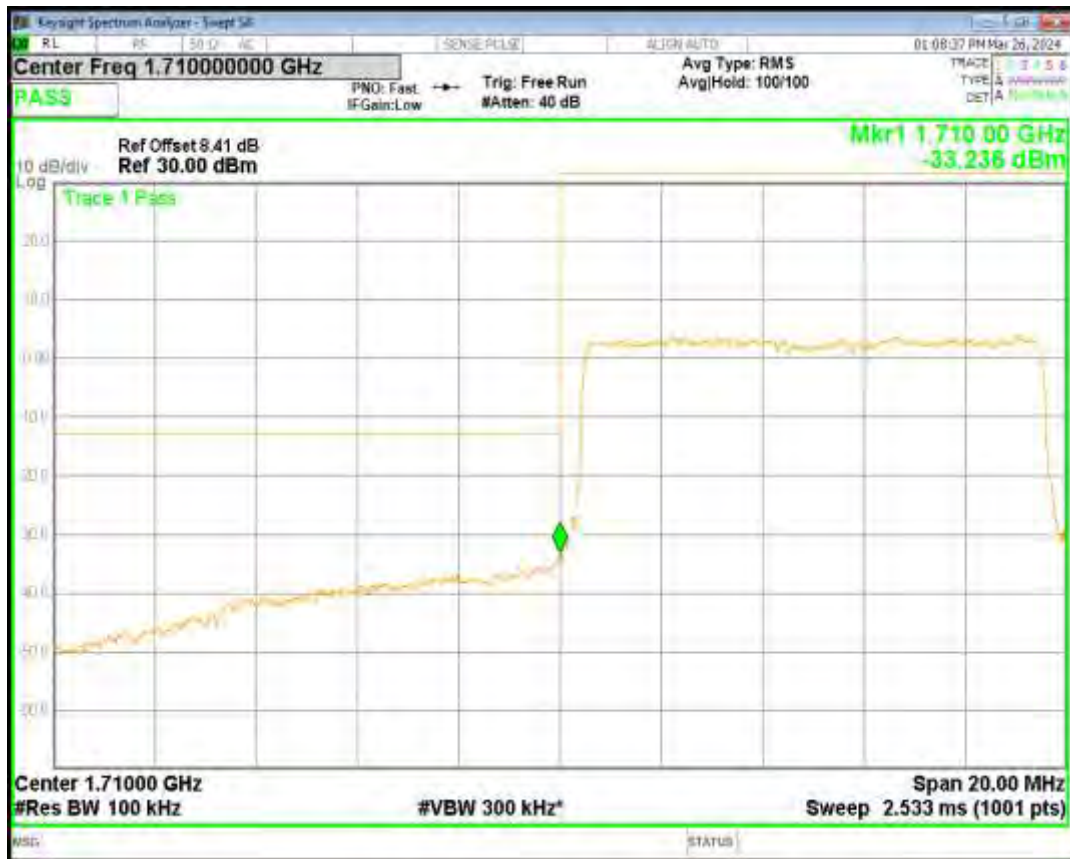
Band4 QPSK BW=10MHz Channel=20350 RB Size=50 Position=#0
