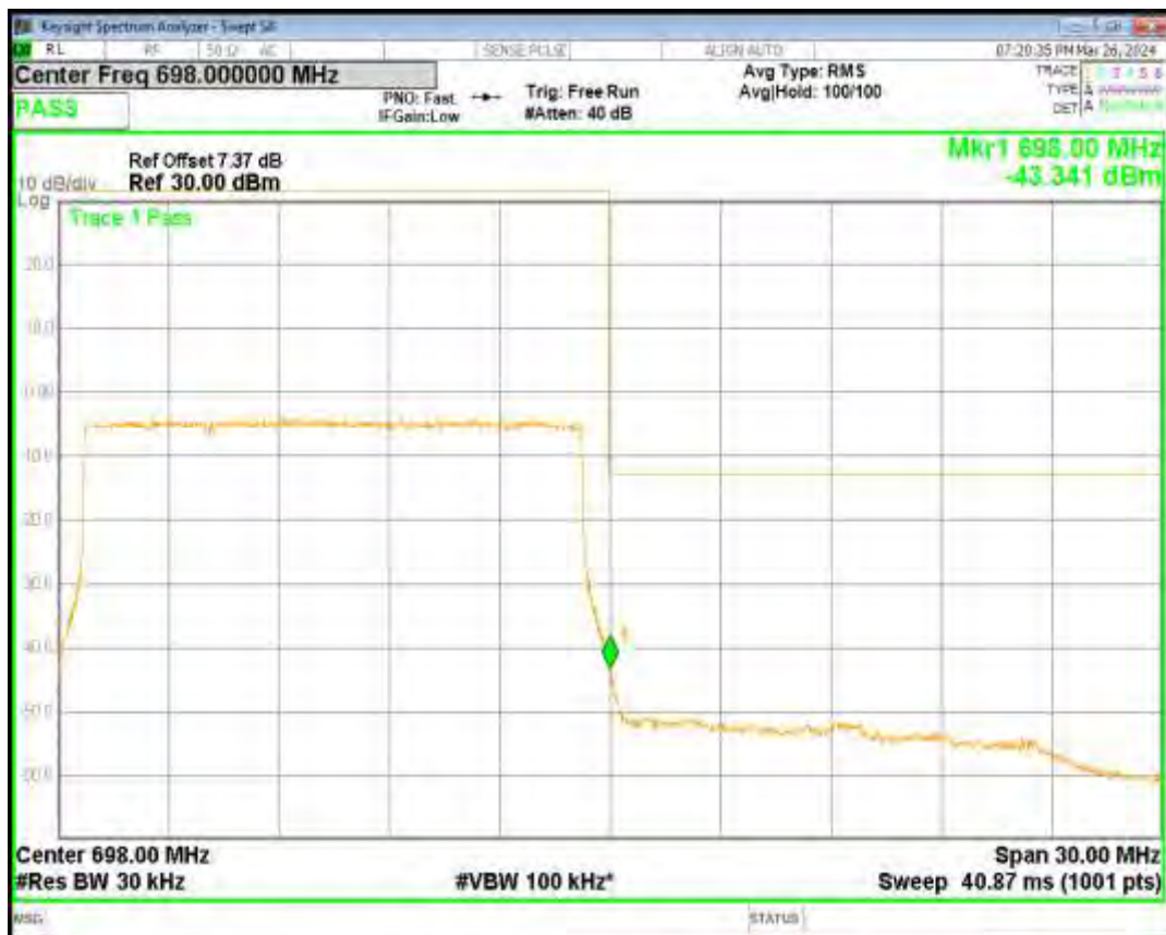
Band71 16QAM BW=20MHz Channel=133222 RB Size=100 Position=#0
