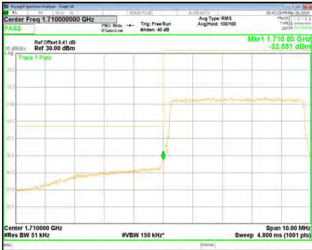
Band66 QPSK BW=15MHz Channel=132047 RB Size=75 Position=#0
