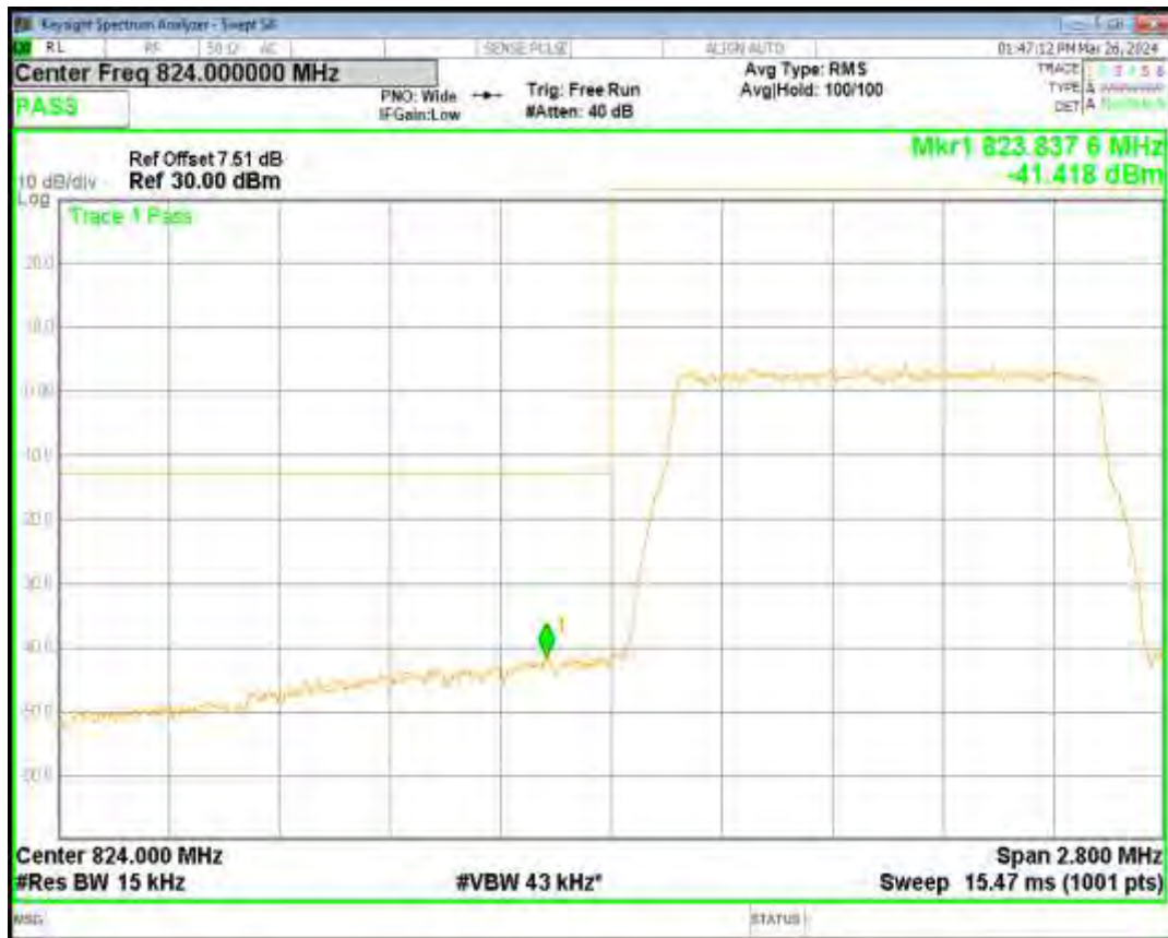
Band5 16QAM BW=1.4MHz Channel=20643 RB Size=6 Position=#0
