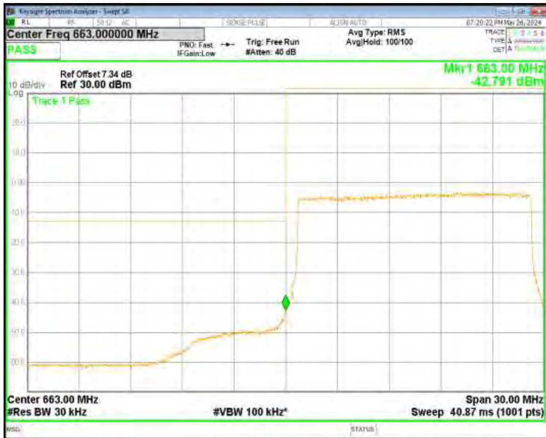
Band71 16QAM BW=15MHz Channel=133397 RB Size=75 Position=#0
