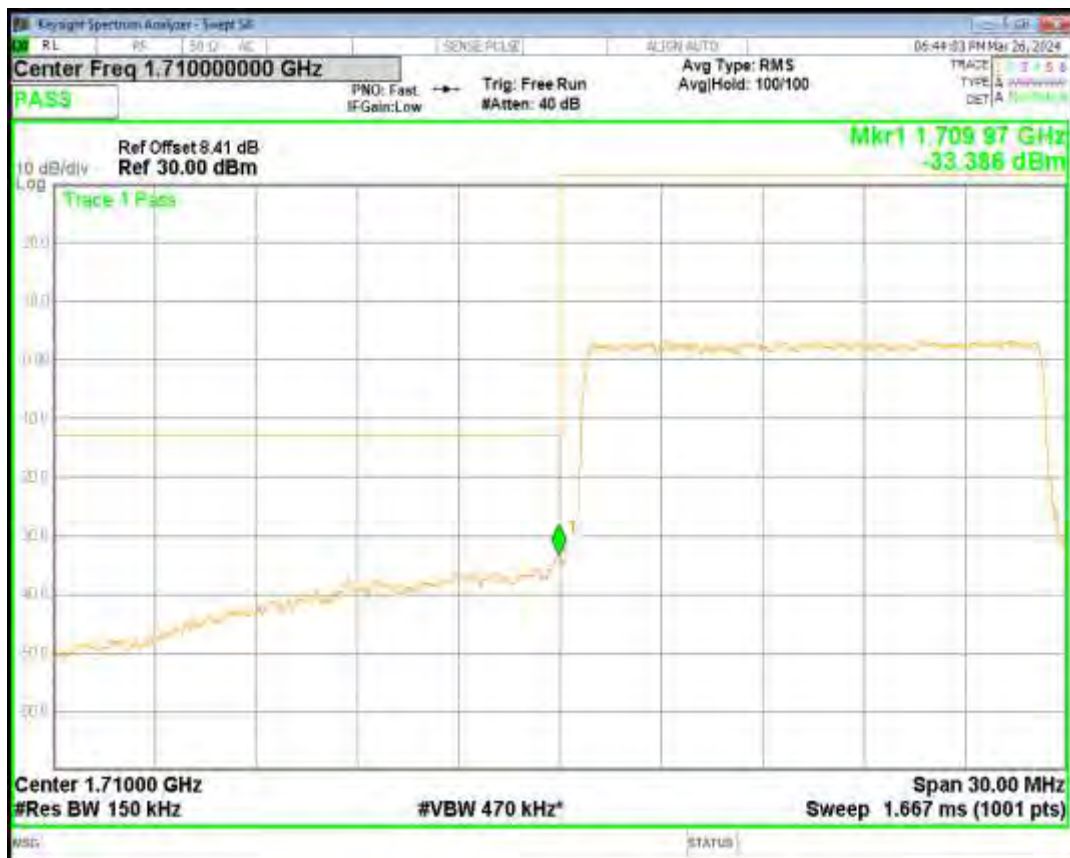
Band66 QPSK BW=15MHz Channel=132597 RB Size=75 Position=#0
