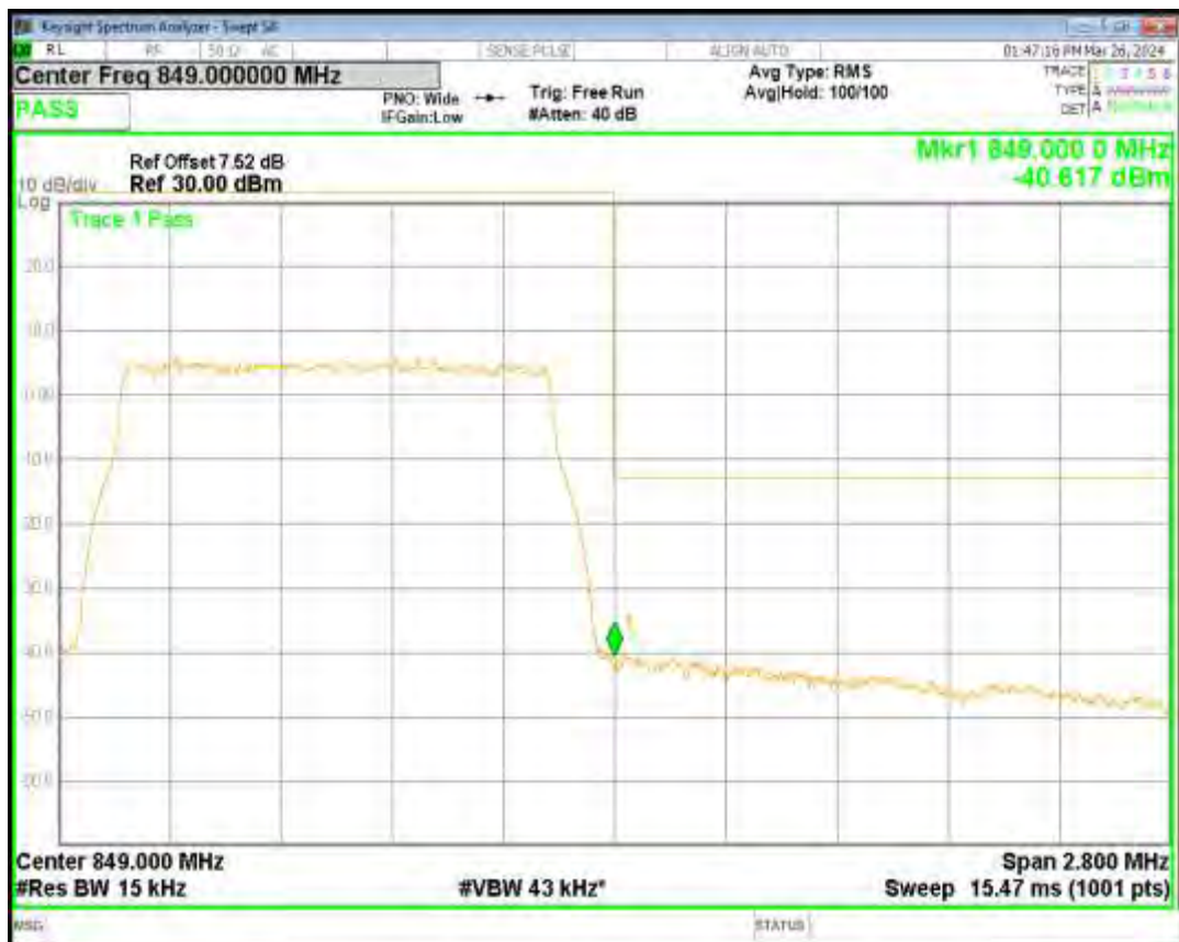
Band5 QPSK BW=10MHz Channel=20450 RB Size=50 Position=#0
