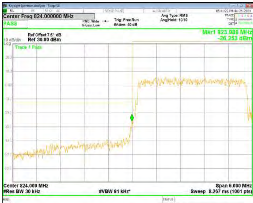
Band26(824-849) QPSK BW=3MHz Channel=27025 RB Size=15 Position=#0
