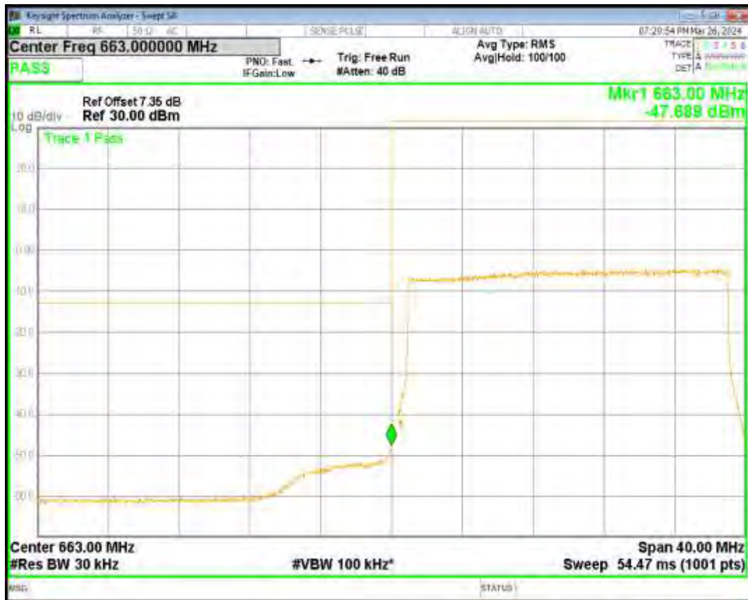
Band71 16QAM BW=20MHz Channel=133372 RB Size=100 Position=#0
