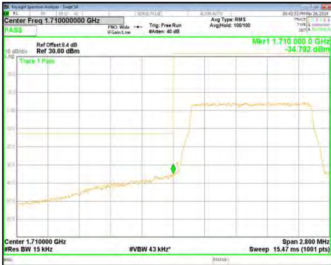
Band66 16QAM BW=5MHz Channel=131997 RB Size=25 Position=#0
