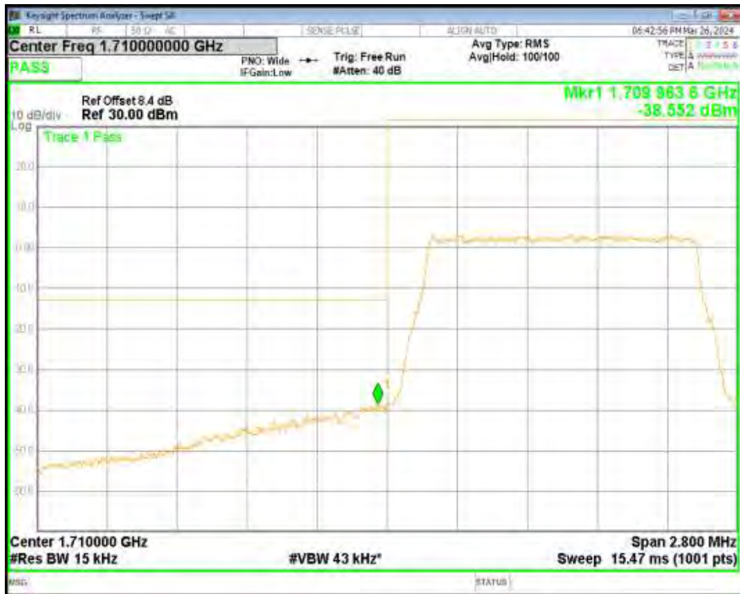
Band66 16QAM BW=1.4MHz Channel=132665 RB Size=6 Position=#0
