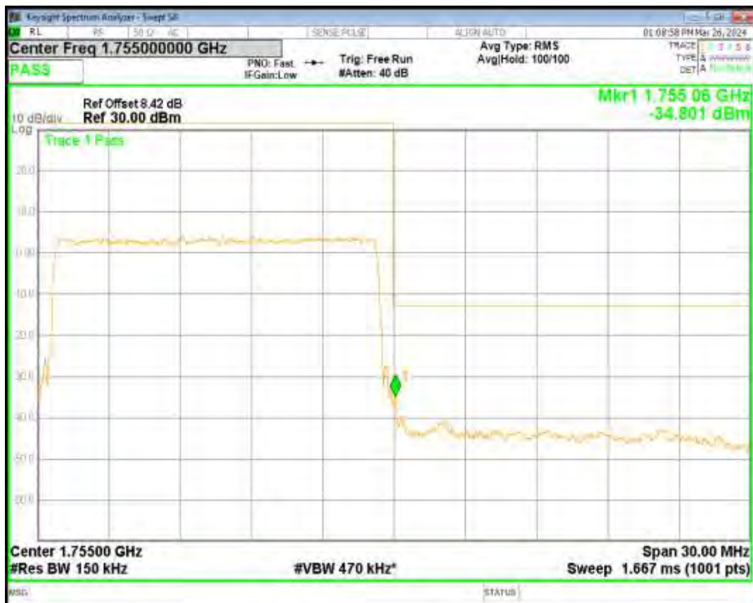
Band4 QPSK BW=20MHz Channel=20050 RB Size=100 Position=#0
