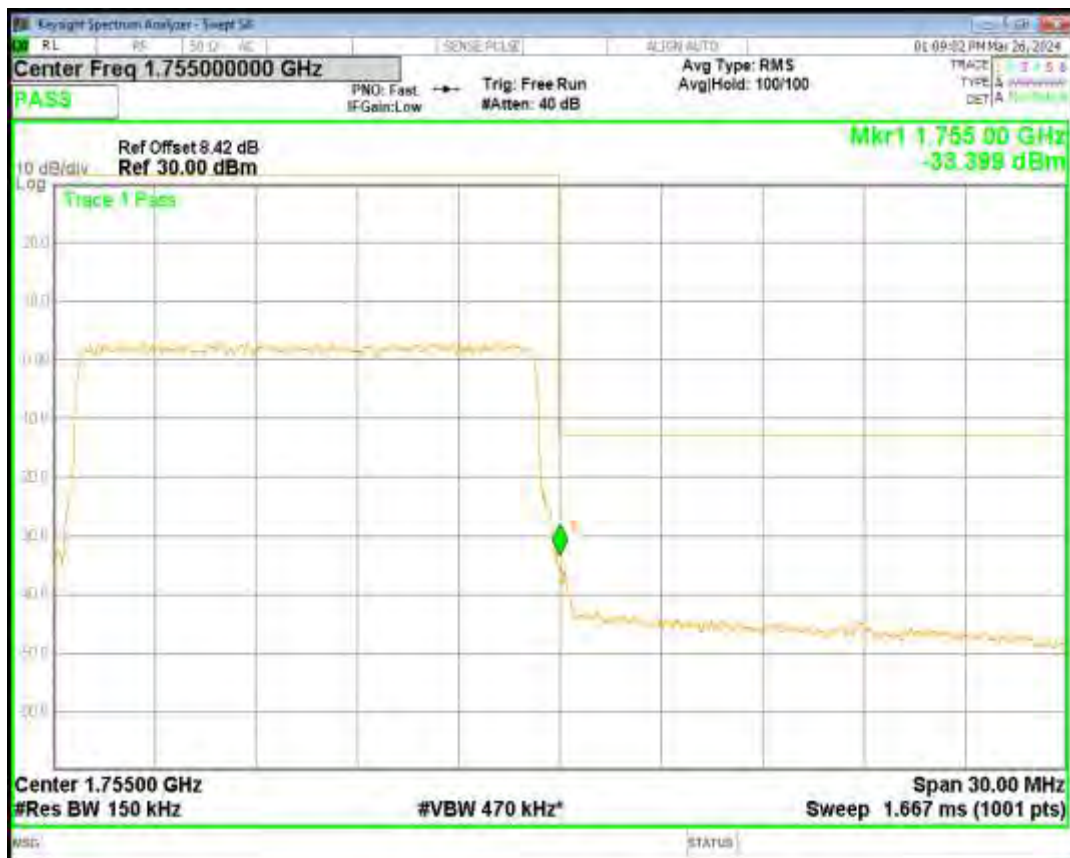
Band4 16QAM BW=3MHz Channel=19965 RB Size=15 Position=#0
