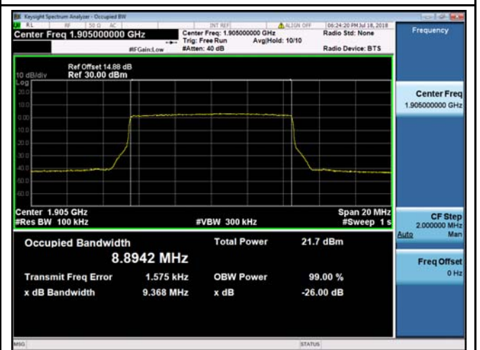
LTE band 2 - Middle CH 16QAM-10
