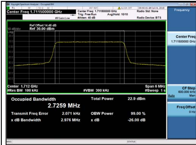
LTE band 4 - Low CH QPSK-3
