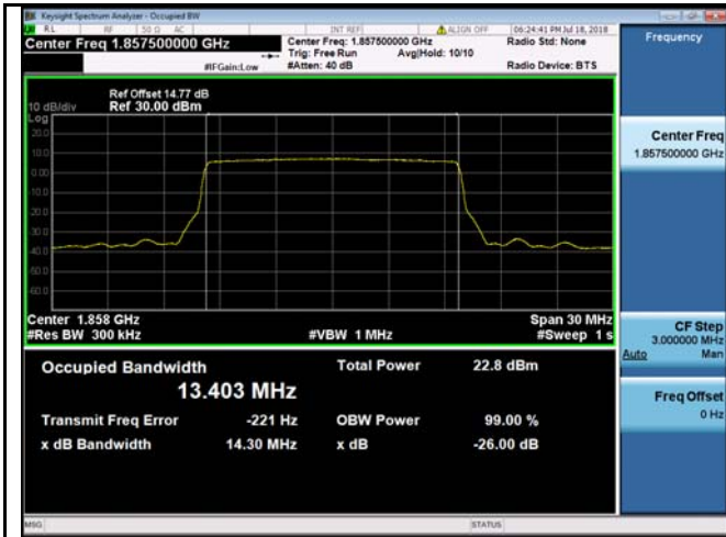
LTE band 2 - Low CH QPSK-15
