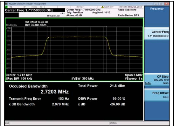
LTE band 4 - Low CH 16QAM-3
