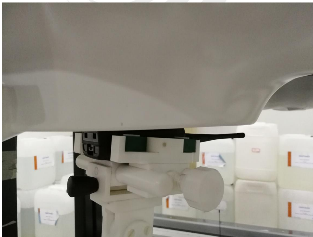
Body Back side(separation distance is 0mm)
