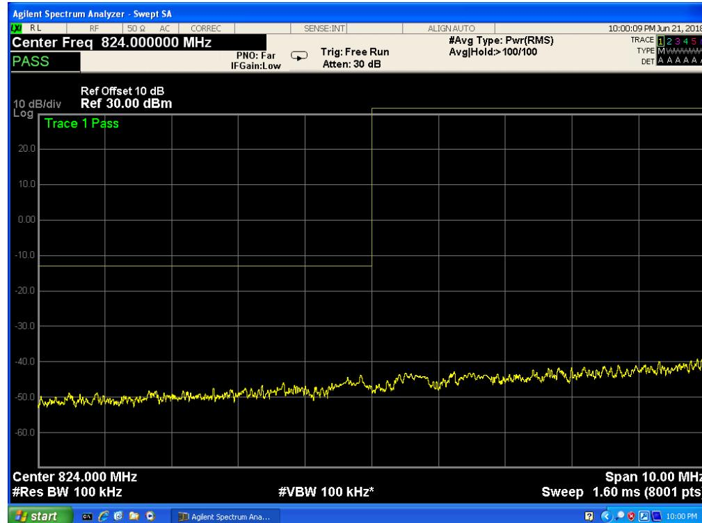
Band 5,UL Channel 20600,UL Frequency 844.0,BW 10.0,NO. RB 50,RB POS. Low,16-QAM
