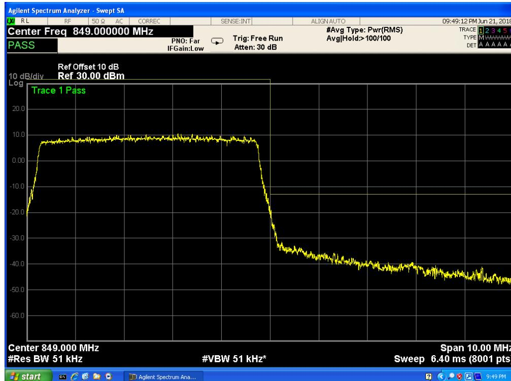
Band 5, UL Channel 20450, UL Frequency 829.0, BW 10.0, NO. RB 50, RB POS. Low, QPSK
