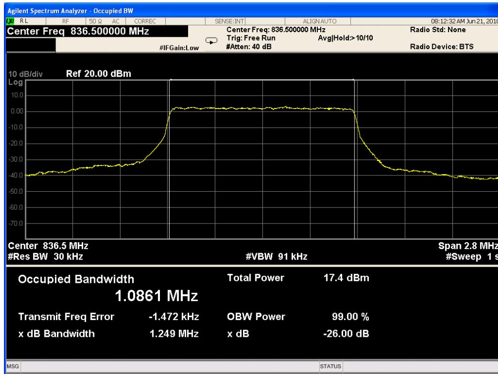
*Band 5, UL Channel 20525, UL Frequency 836.5, BW 1.4, NO. RB 6, RB POS. Low, 16-QAM*
