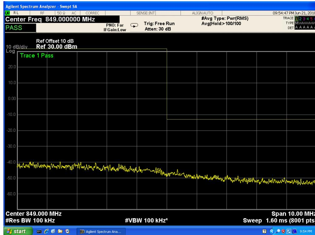
Band 5, UL Channel 20600, UL Frequency 844.0, BW 10.0, NO. RB 50, RB POS. Low, QPSK
