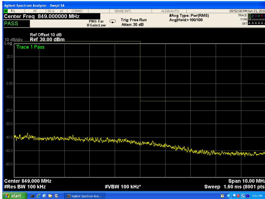
Band 5,UL Channel 20450,UL Frequency 829.0,BW 10.0,NO. RB 50,RB POS. Low,16-QAM
