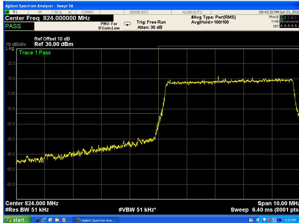
Band 5, UL Channel 20425, UL Frequency 826.5, BW 5.0, NO. RB 25, RB POS. Low, 16-QAM
