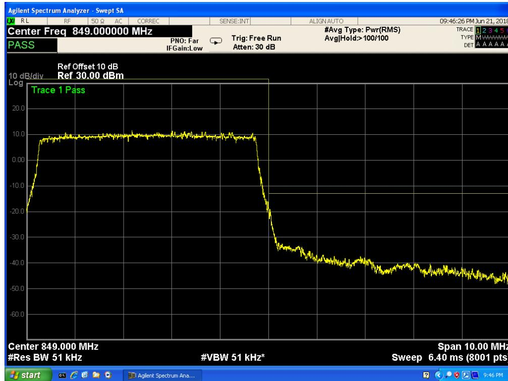
Band 5, UL Channel 20625, UL Frequency 846.5, BW 5.0, NO. RB 25, RB POS. Low, 16-QAM
