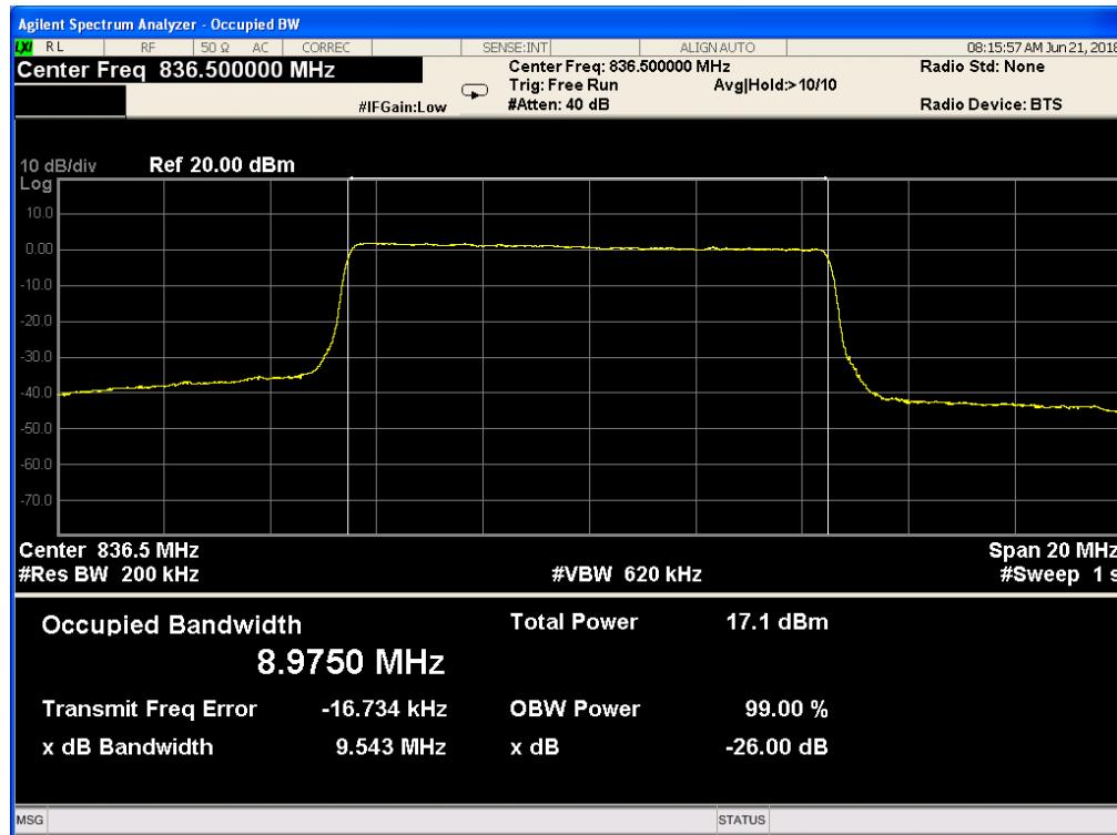
**Band 5, UL Channel 20525, UL Frequency 836.5, BW 10.0, NO. RB 50, RB POS. Low, 16-QAM**
