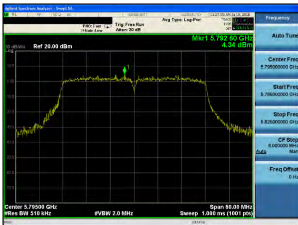
(802.11ac40) PSD plot on channel 159
