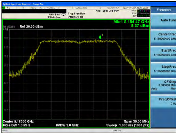
(802.11a) PSD plot on channel 40
