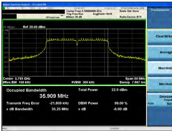
(802.11 n40) 6dB Bandwidth plot on channel 159
