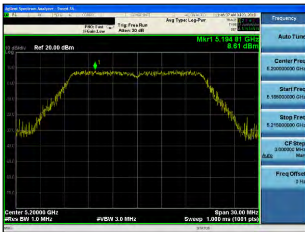
(802.11a) PSD plot on channel 48
