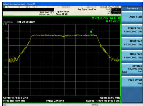
(802.11ac20) PSD plot on channel 165
