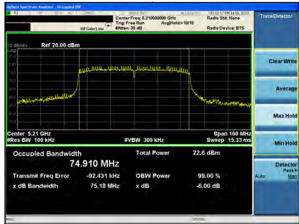
(802.11 ac80) 6dB Bandwidth plot on channel 42
