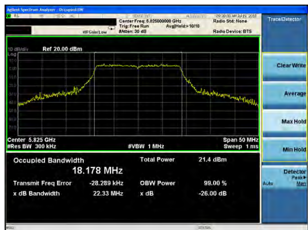
(802.11 n20) -26dB&99%Bandwidth plot on channel 165
