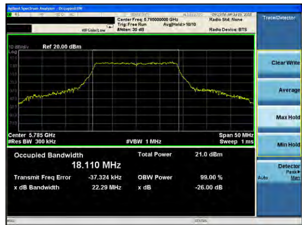
(802.11 ac20) -26dB&99%Bandwidth plot on channel 165
