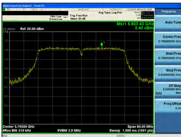
(802.11n40) PSD plot on channel 159
