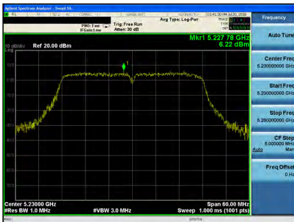
(802.11ac40) PSD plot on channel 46
