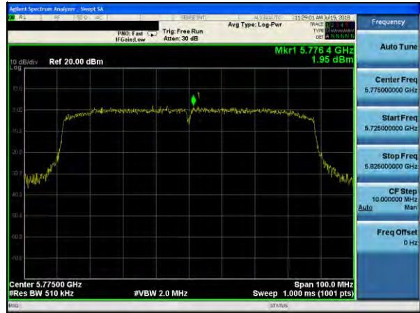
(802.11ac80) PSD plot on channel 155
