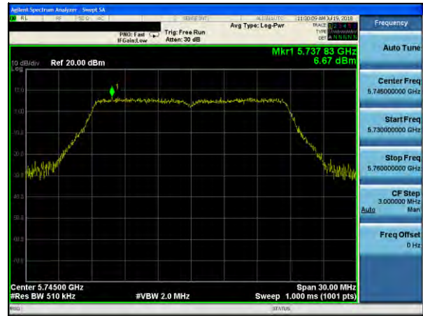
(802.11n20) PSD plot on channel 157
