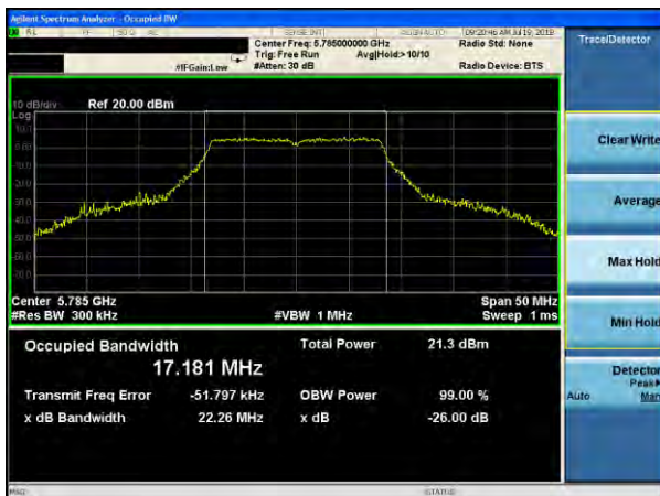
(802.11a) -26dB&99%Bandwidth plot on channel 165
