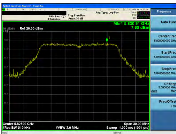
(802.11a) PSD plot on channel 165
