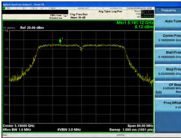
(802.11n40) PSD plot on channel 46
