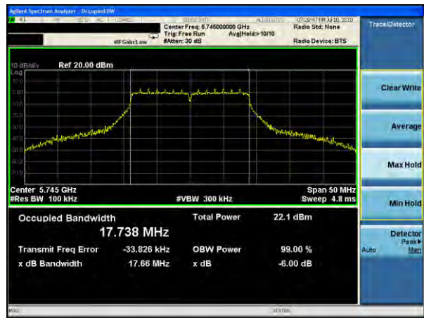
(802.11 n20) 6dB Bandwidth plot on channel 157
