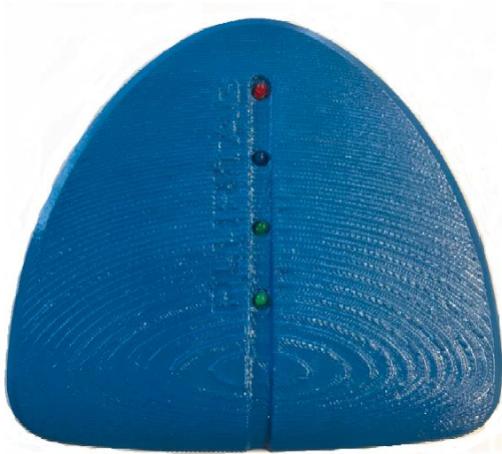
Figure 1-1 TOF RTLS Reader
