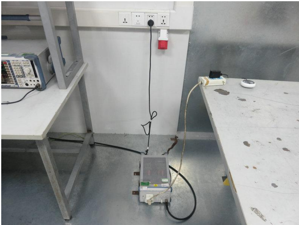
Photo of Conducted Emission Measurement
