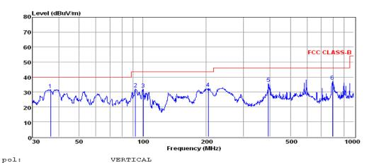
Freq Reading CabLos Antfac Measured Limit Over Remark MHz dBuV dВ dB/m dBuV/m dBuV/m dВ -8.37 18.50 0.41 12.72 31.63 40.00 36.64 2 92.46 19.34 0.56 12.36 32.26 43.50 -11.24 3 100.58 18.25 0.60 13.11 31.96 43.50 -11.54 QP 4 204.24 20.70 0.99 10.70 32.39 43.50 -11.11 QP
