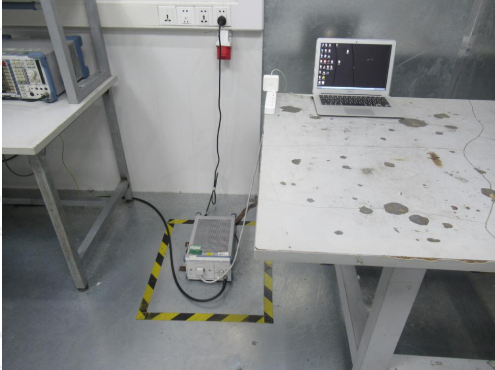
Photo of Conducted Emission Test
