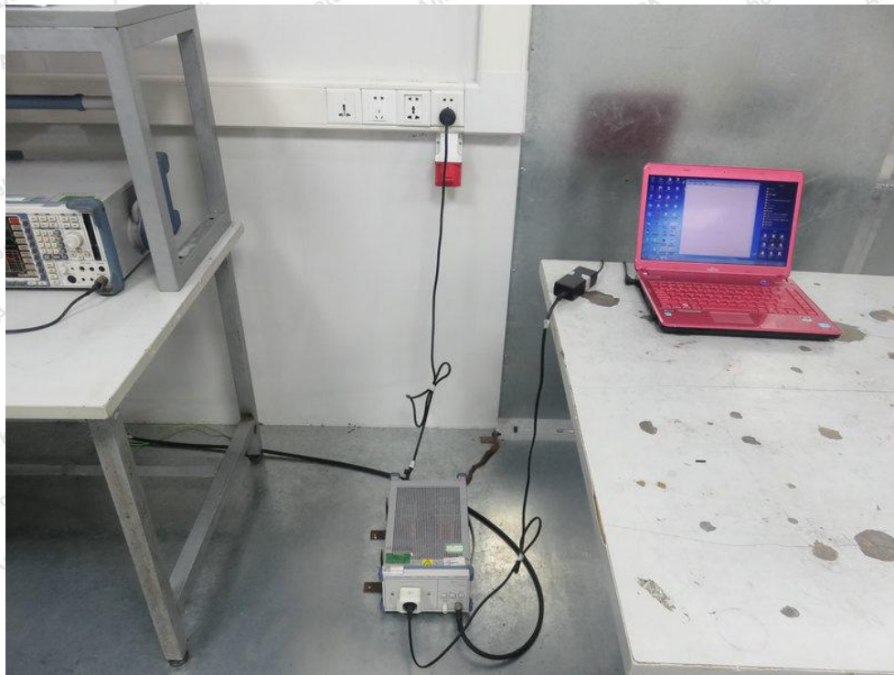
Photo of Conducted Emission Measurement
