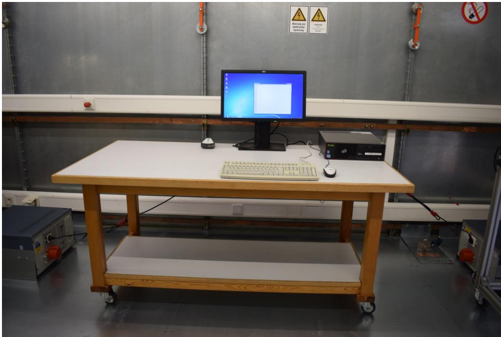
Picture 5: Test setup AC power line conducted emissions (front view)
