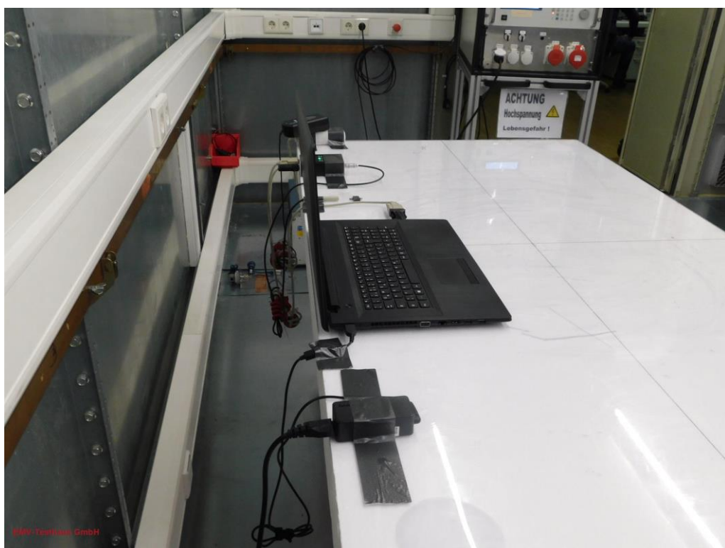
Picture 8: Test setup AC power line conducted emissions (rear view)
