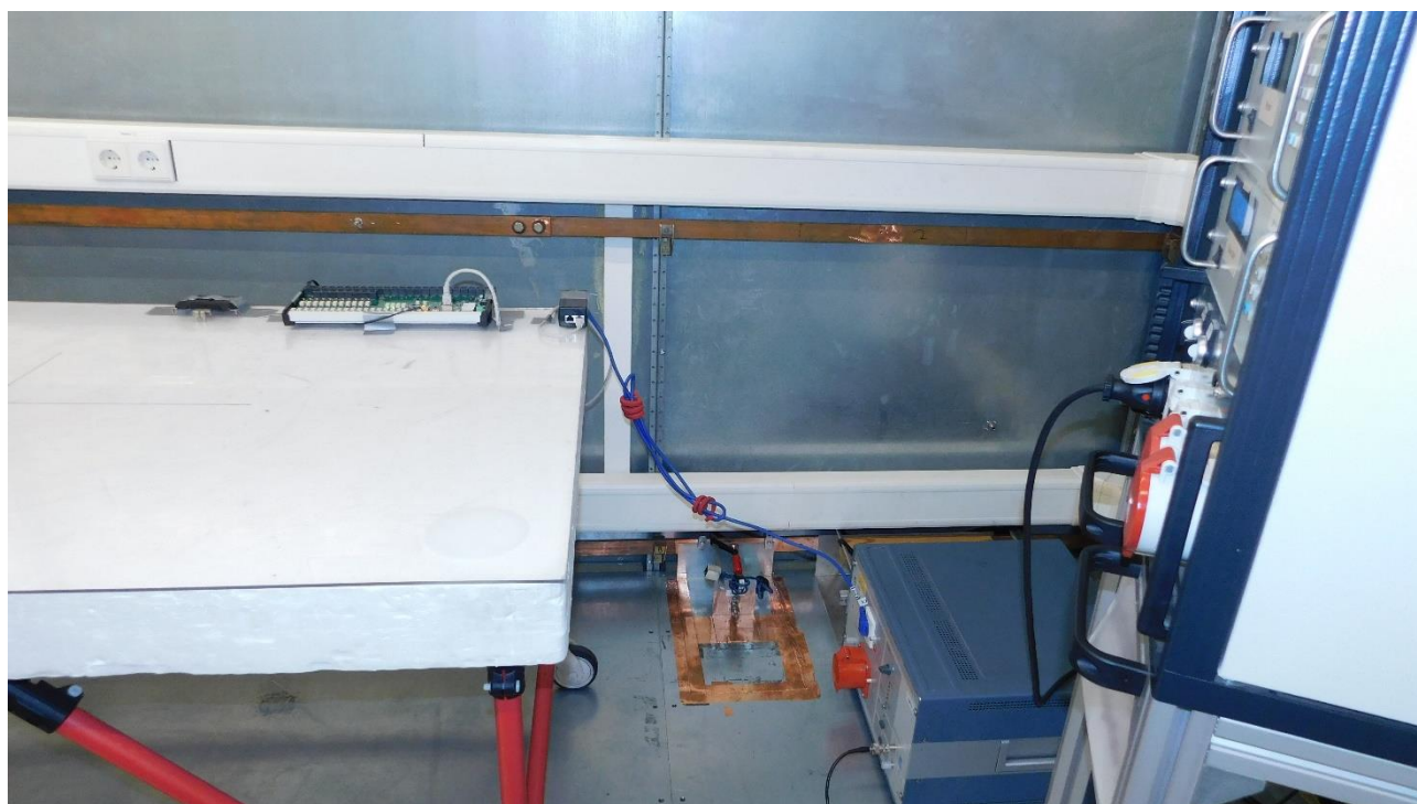
Picture 7: Test setup AC power line conducted emissions (front view)
