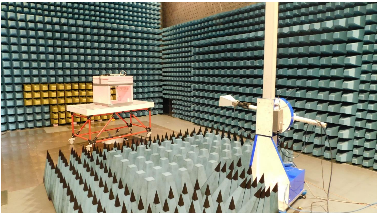
Picture 6: SAC, radiated emission test 1 GHz – 2 GHz (rear view)
