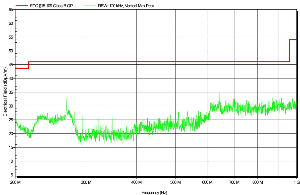
**Radiated emissions under normal conditions according to FCC Part 15b**
