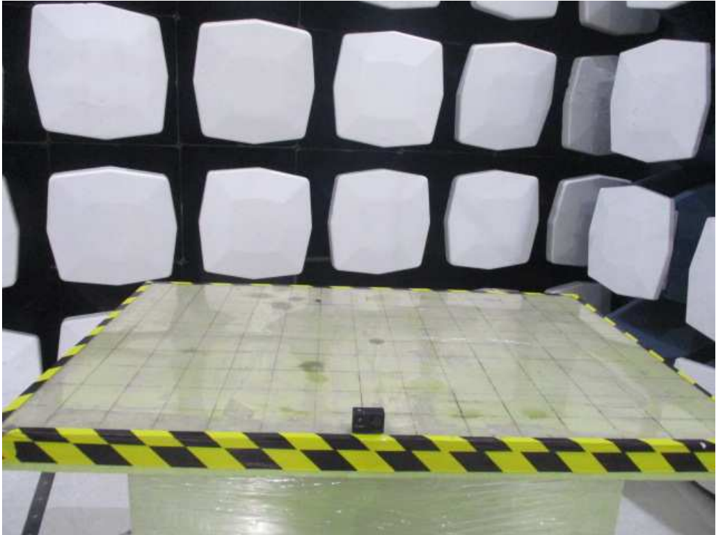
Radiated Emissions up to 1GHz (Placed at the center of the turntable)
