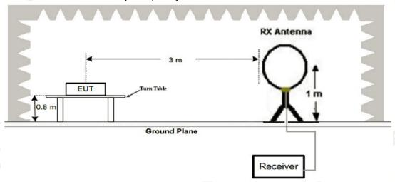
2. Radiated Emission Test-Up Frequency 30MHz~1GHz
