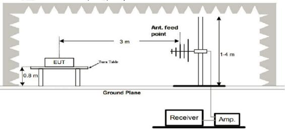
3. Radiated Emission Test-Up Frequency Above 1GHz
