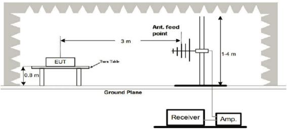
3. Radiated Emission Test-Up Frequency Above 1GHz
