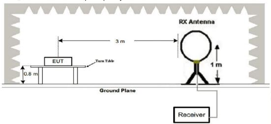
2. Radiated Emission Test-Up Frequency 30MHz~1GHz
