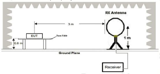
2. Radiated Emission Test-Up Frequency 30MHz~1GHz
