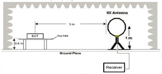
2. Radiated Emission Test-Up Frequency 30MHz~1GHz
