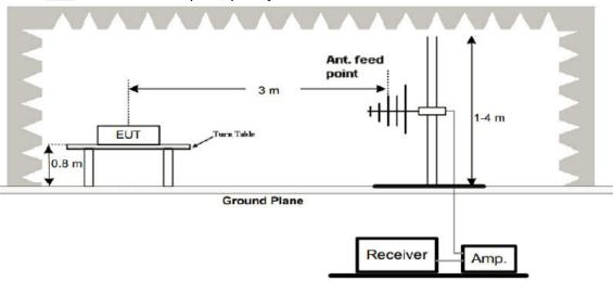
3. Radiated Emission Test-Up Frequency Above 1GHz
