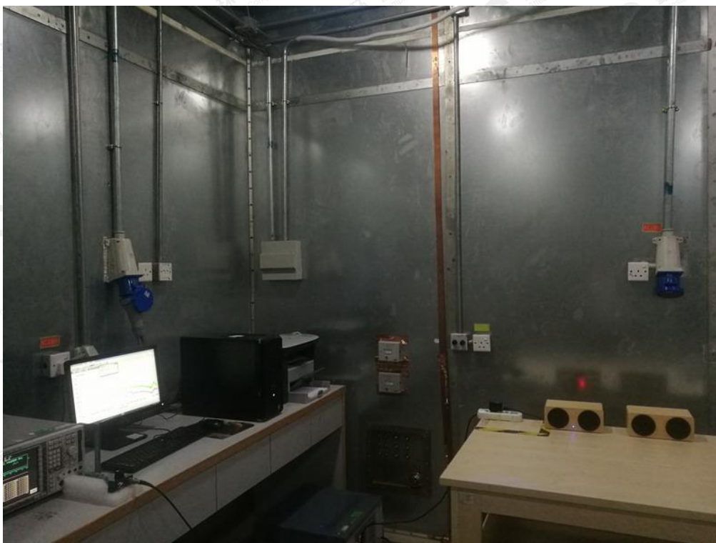
FCC RADIATED EMISSION TEST SETUP
