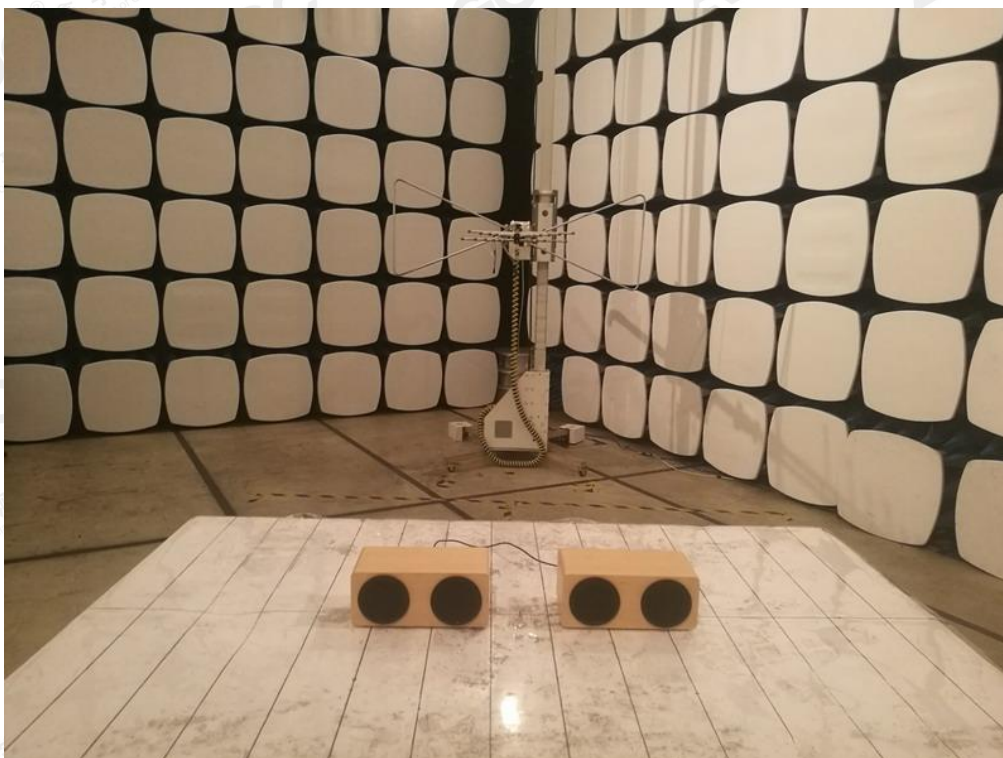
FCC RADIATED EMISSION TEST SETUP
