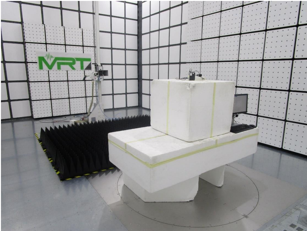
Description: Radiated Emission Test Setup for 1GHz~18GHz
