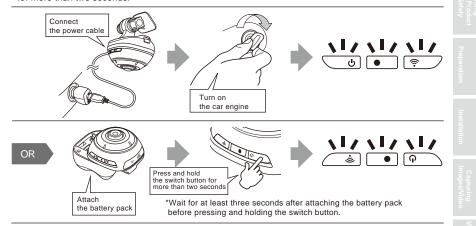
\*The camera body will begin updating automatically a few seconds after the camera body is switched on. During this update, all LEDs except the memory LED will start blinking in red.
