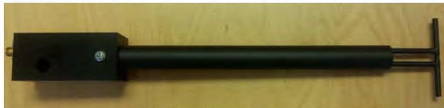
Figure 1 – MVG COMOSAR Validation Dipole
