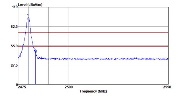
Mode:b; Polarization:Vertical; Modulation:GFSK; ; Channel:High
