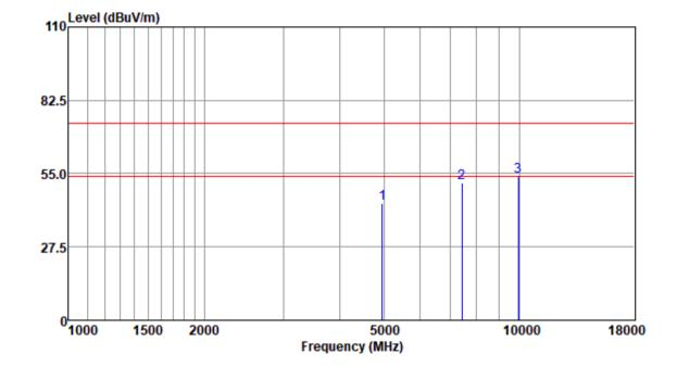
Mode:b; Polarization:Horizontal; Modulation:GFSK; ; Channel:High
