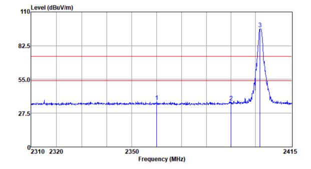
Mode:b; Polarization:Horizontal; Modulation:GFSK; ; Channel:Low
