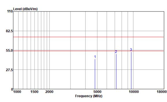
Mode:b; Polarization:Vertical; Modulation:8DPSK; ; Channel:Low
