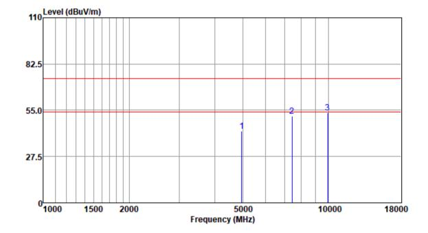
Mode:b; Polarization:Vertical; Modulation:GFSK; ; Channel:High
