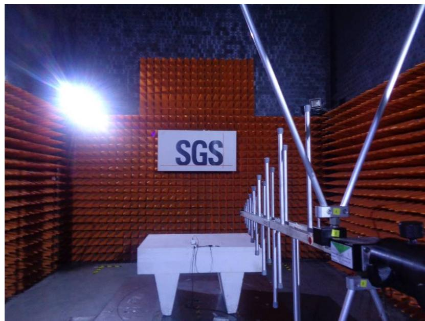
**7.3 Radiated Emissions (above 1GHz) Test Setup**
