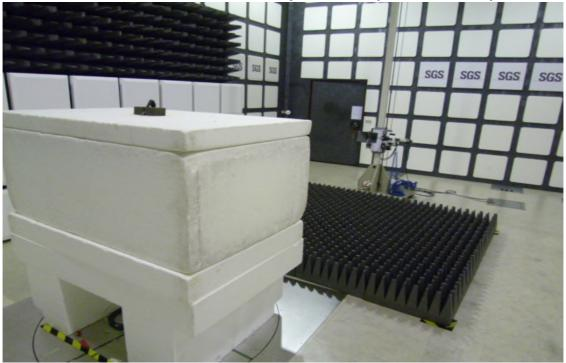
Radiated Emission Set up Photos (Front View)
