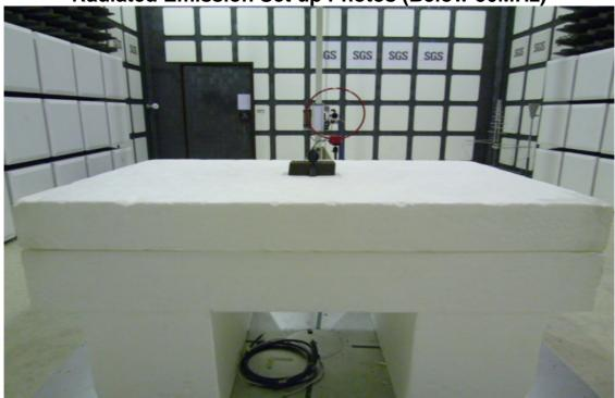
Radiated Emission Set up Photos (Below 1GHz)
