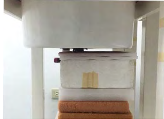
Fig.3 EUT Back side to flat phantom
