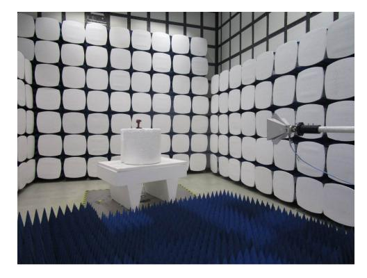
1.3 Radiated Emissions Test Setup
