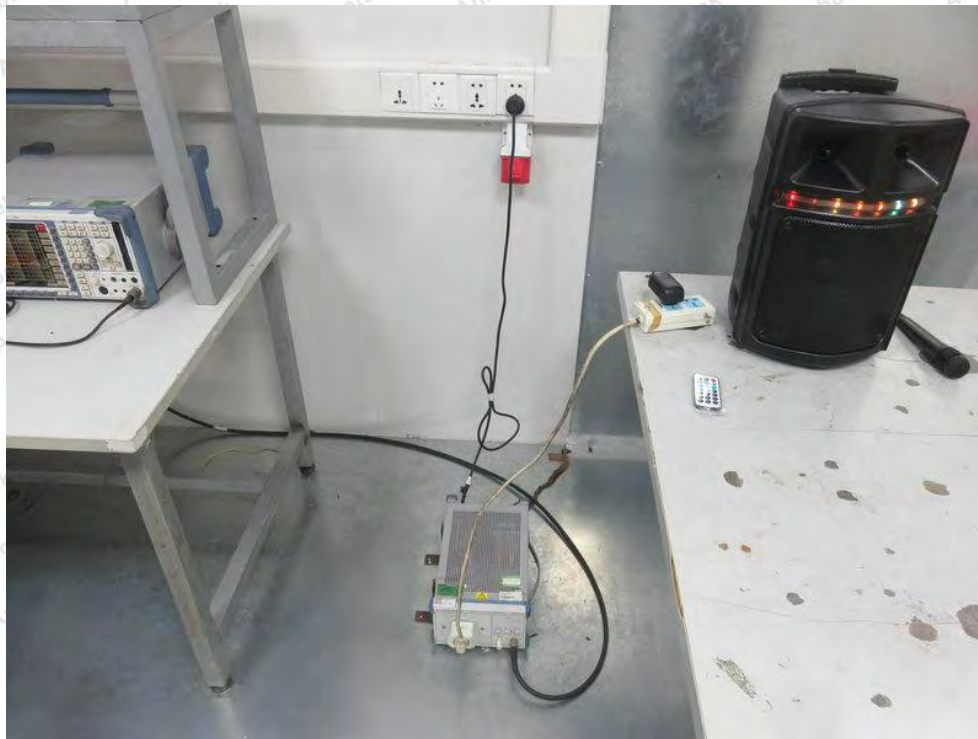
Photo of Conducted Emission Measurement
