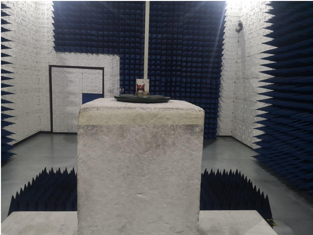
RADIATED EMISSION TEST SETUP ABOVE 1GHZ
