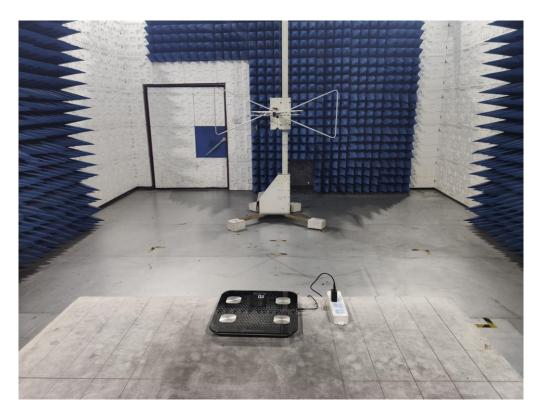
RADIATED EMISSION TEST SETUP ABOVE 1GHZ
