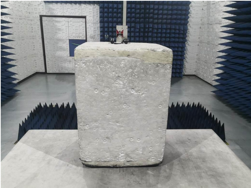
RADIATED EMISSION TEST SETUP ABOVE 1GHZ
