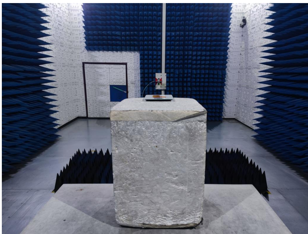
RADIATED EMISSION TEST SETUP ABOVE 1GHz
